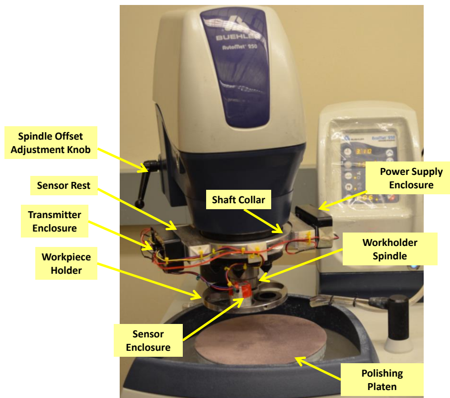
Fig. 2: Buehler Automet ® 250 experimental CMP polishing setup showing the sensor arrangement and various machine elements.
