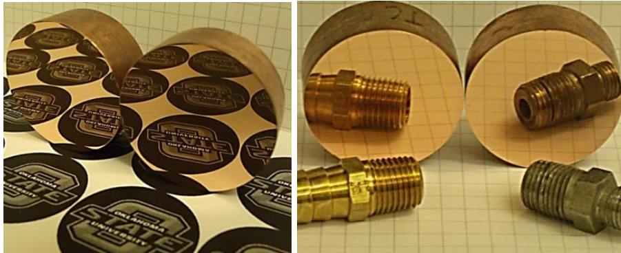
Figure 4-51: Blanket copper wafers after 9 minutes of CMP with 70 nm colloidal silica slurry.
