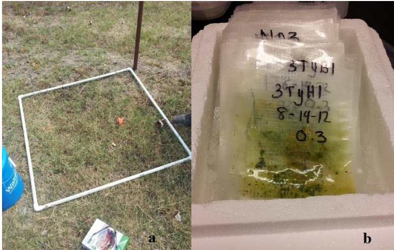
Figure. 1. A) One square meter quadrat used to sample sites along transects; b) macerated plant samples placed on ice.
