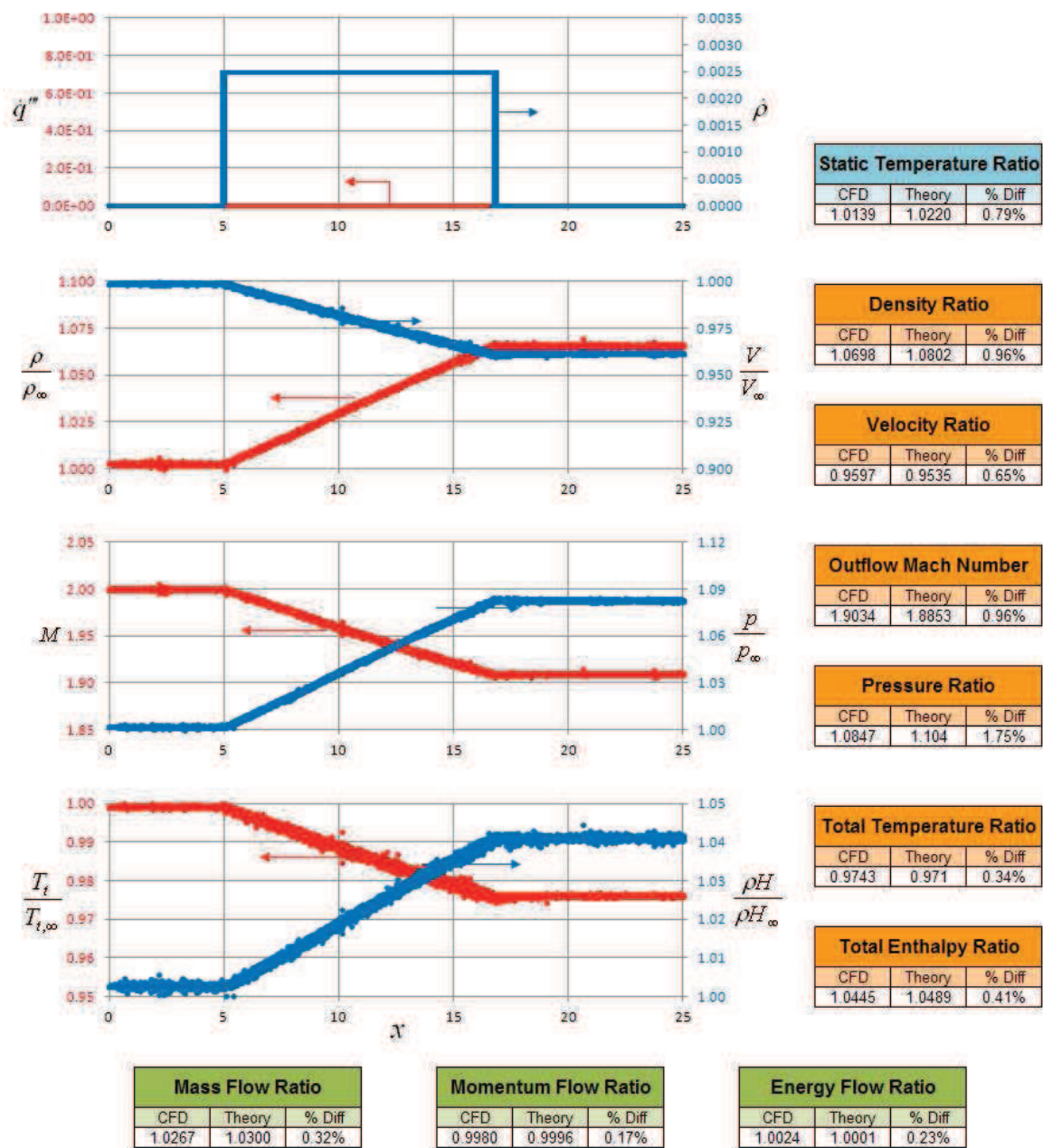
Figure 7.67: Supersonic (Mach 2.0) Constant Mass Generation.
