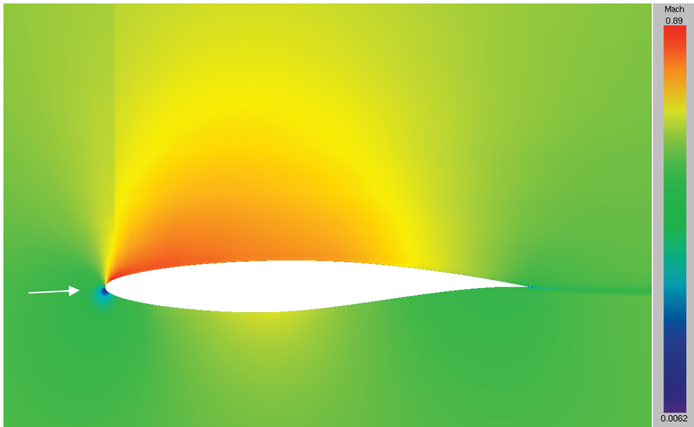
Figure 7.9: Mach Distribution around RAE 2822 Airfoil (Mach 0.6).
