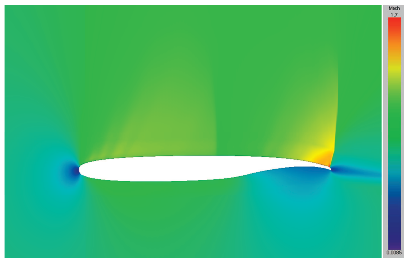
Figure 7.34: Mach Distribution around NASA 10% Supercritical Airfoil (CFDsol).
