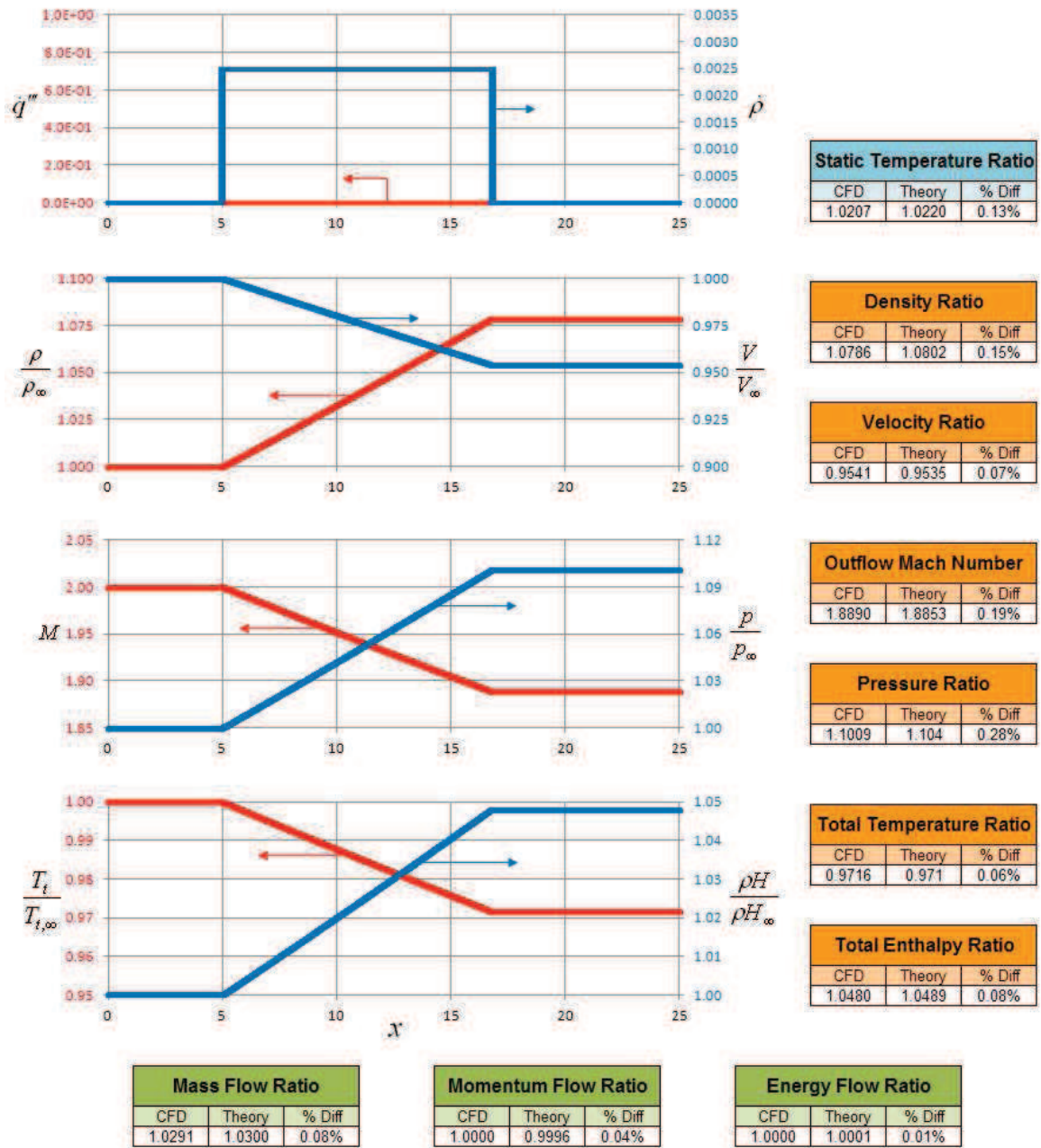
Figure 6.77: Supersonic (Mach 2.0) Constant Mass Generation.
