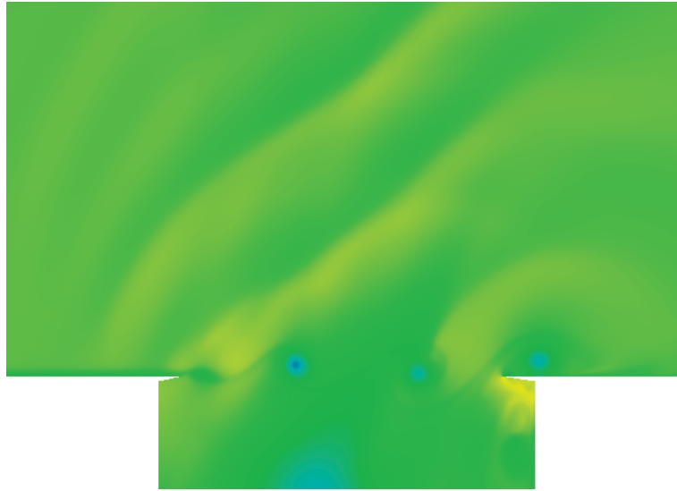
Figure 6.140: Acoustic Waves above Lipped Cavity (Density, NS2D).
