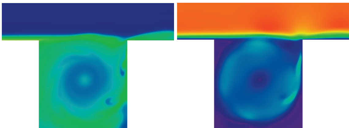
Figure 6.134: Entropy (left) and Velocity (right) in Square Cavity ( L:D = 1:1 ).
