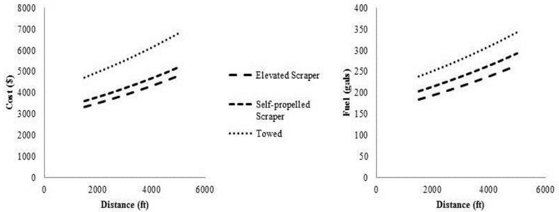
Figure 4.32. Economic and energy impact of scraper based on scraper type and distance
