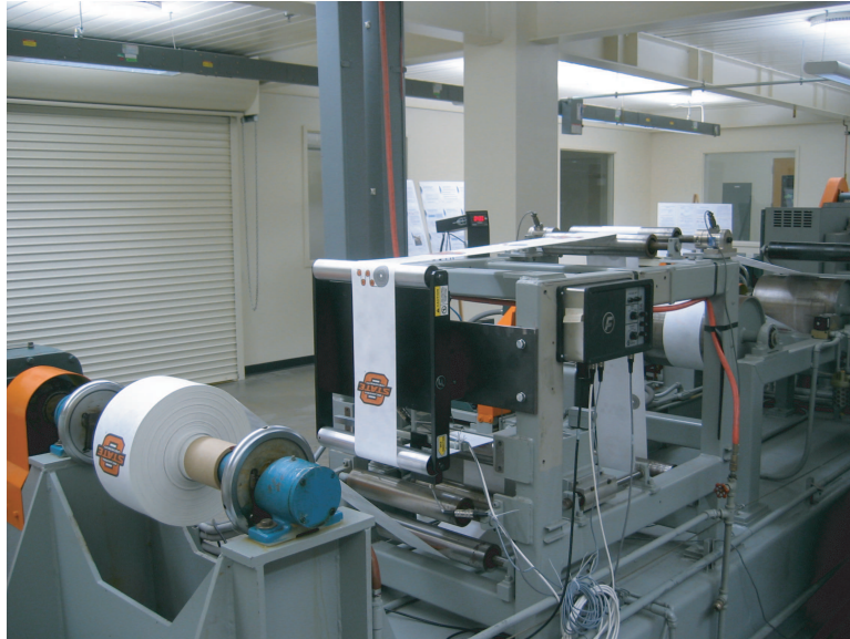
Figure 1.1: The Euclid Web Line (EWL), Web Handling Research Center.
