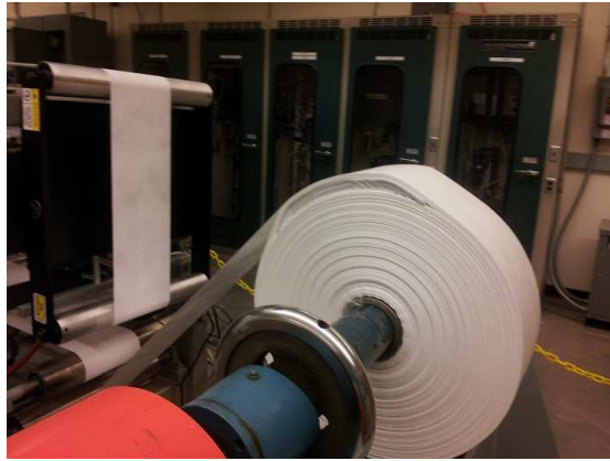
(a) Roll with a flattened bulge.
