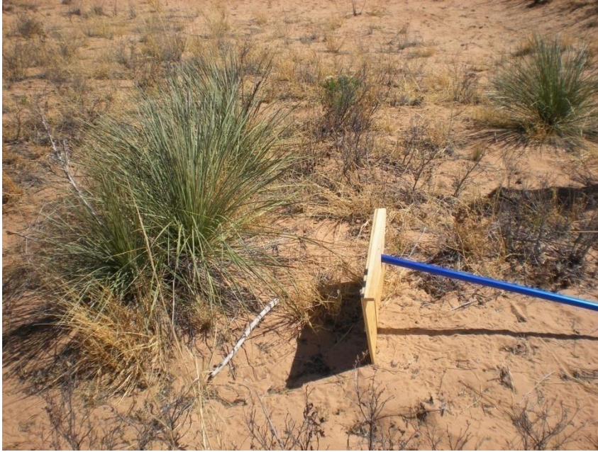
Figure 2.1: The custom-designed mirror on a pole used to elicit territorial aggression. The pole is telescopic (2-4 m) and made of lightweight aluminum.
