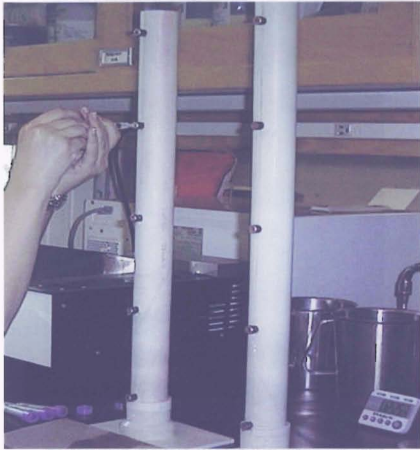
Fig. 4.3 Settling columns (65 cm in height) built of PVC with seals at 15 cm intervals for removing samples.
