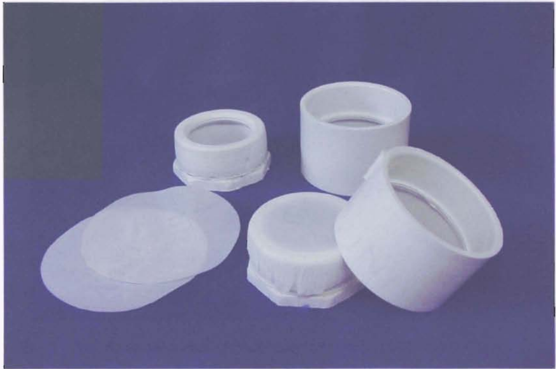
Fig. 3.4 Spore cages made of PVC couplers and reducers with Nitex mesh.
