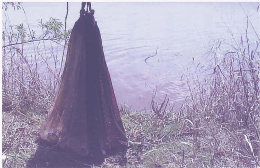
Fig 3.5 Field survival sampling method using mesh utility bags and spore cages.
