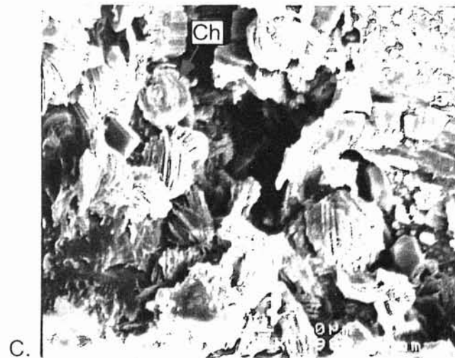
Figure 27. A. Scanning electron photomicrograph (SEM) Pore bridging smectite (S) and illite (I) coating grains. Kaolinite (K) filling pore space. Detrital quartz (Q) grain. B. Kaolinite (K) filling pore space. C. Chlorite (CH) pore filling.
