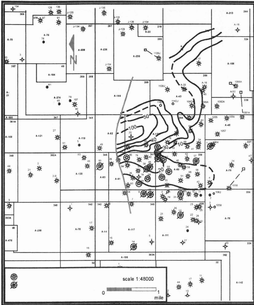
Figure 13. Isopach map showing the prograding deltaic nature of the 10250 ft. Lower Vicksburg interval.
