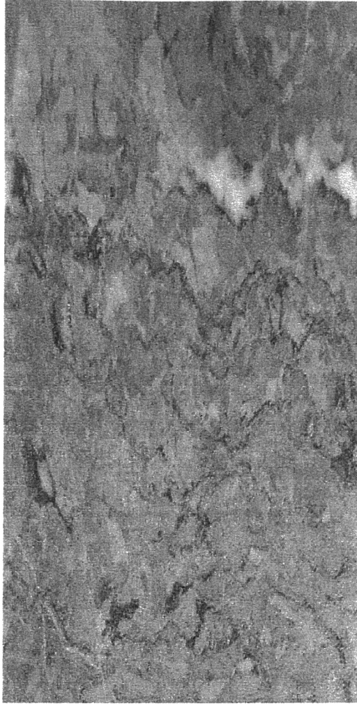
Fig. 29. Core photo of the L. L. Tontz #1 at 4978 feet showing fracture and vug filling by milky white calcite. Much of the porosity found in this core is accounted for at around this depth due to unfilled or partially unfilled fractures and vugs.
