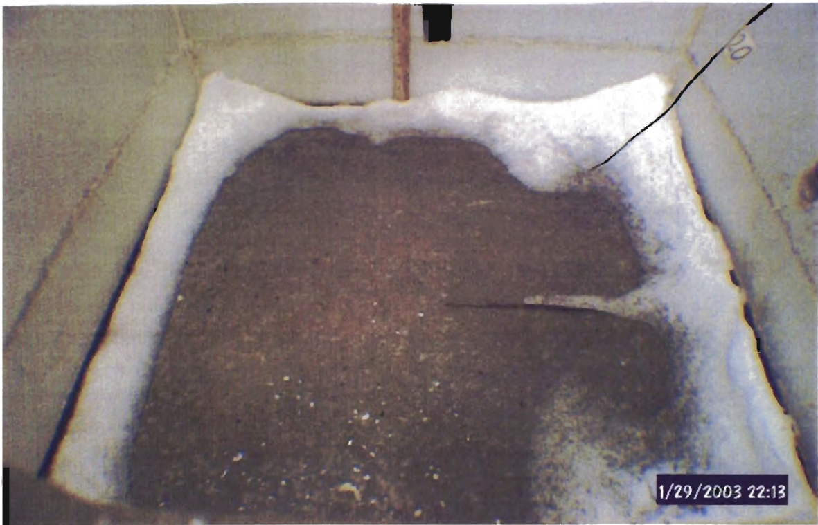
Figure 4.5-19: FD-RG Predicted Snow Free Area Ratio 1.00, measured: 0.95
