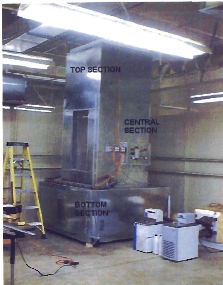
Figure 3.3-8: Environmental chamber sections
