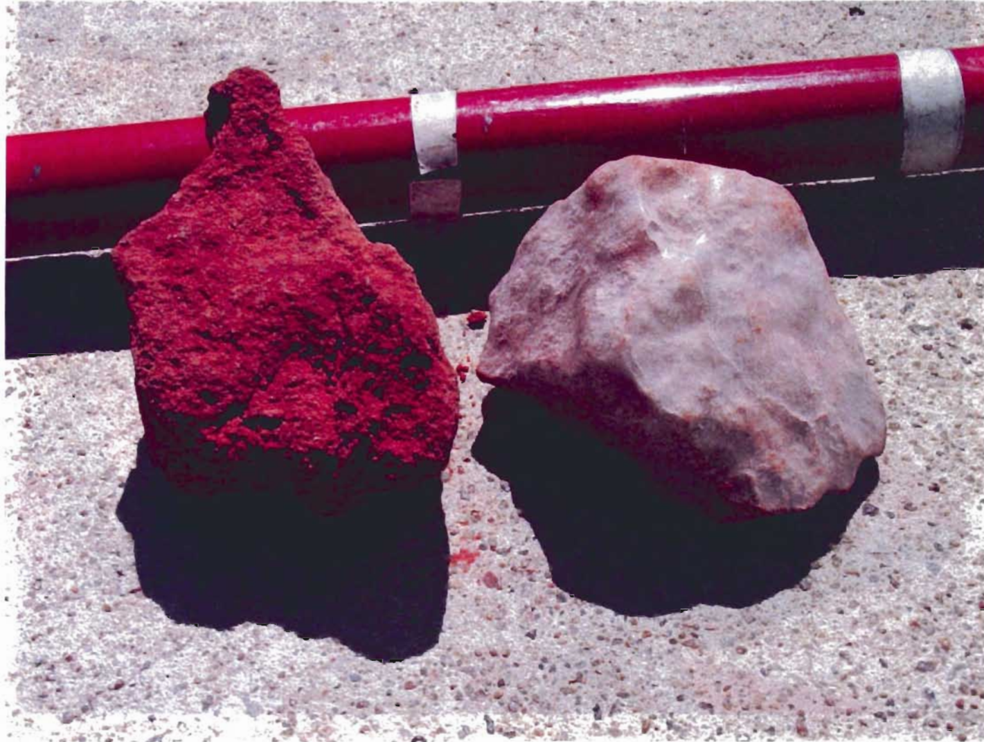
Hand samples of sandstone from the White Horse Group. The sample on the right is coated with paraffin (Scale = 10cm between white bands).
