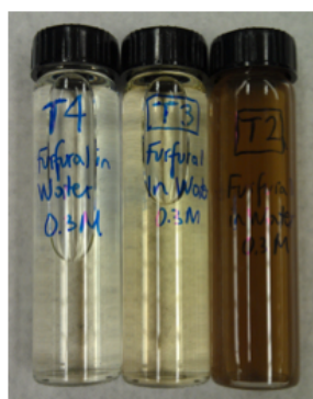
Figure 6.3. Products from furfural thermal stability test. Temperature of the test, from left to right, was: 50°C, 150°C and 250°C.
