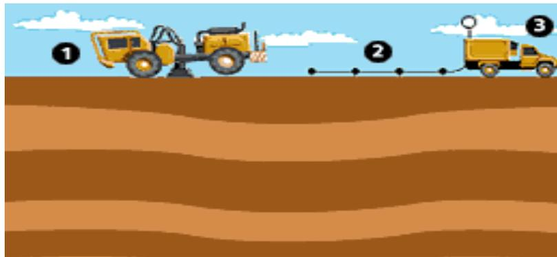
**Figure 1.3:** Modern-day oil prospectors use sound waves to locate oil. In one technique, (1) a signal is sent into the rock by a vibrator truck, (2) the reflected waves are received by geophones, and (3) the data is transmitted to a laboratory truck.
