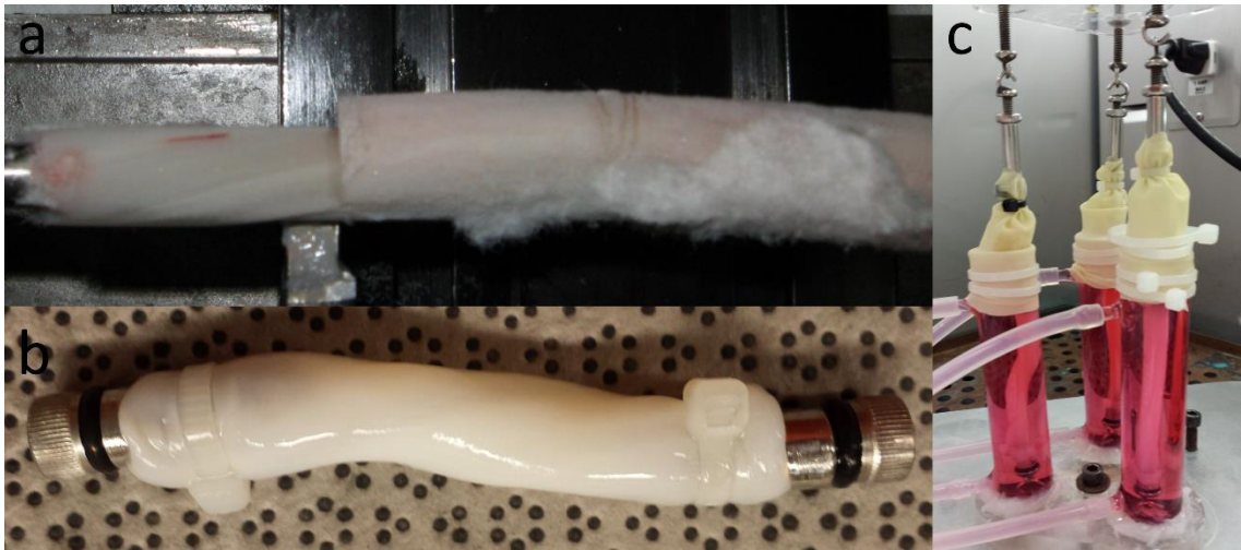
Figure 5.1: a) A partially lathed umbilical cord exposing the HUV. b) Image of an HUV seeded with collagen gel/MSCs. c) Constructs cultured within the bioreactor.
