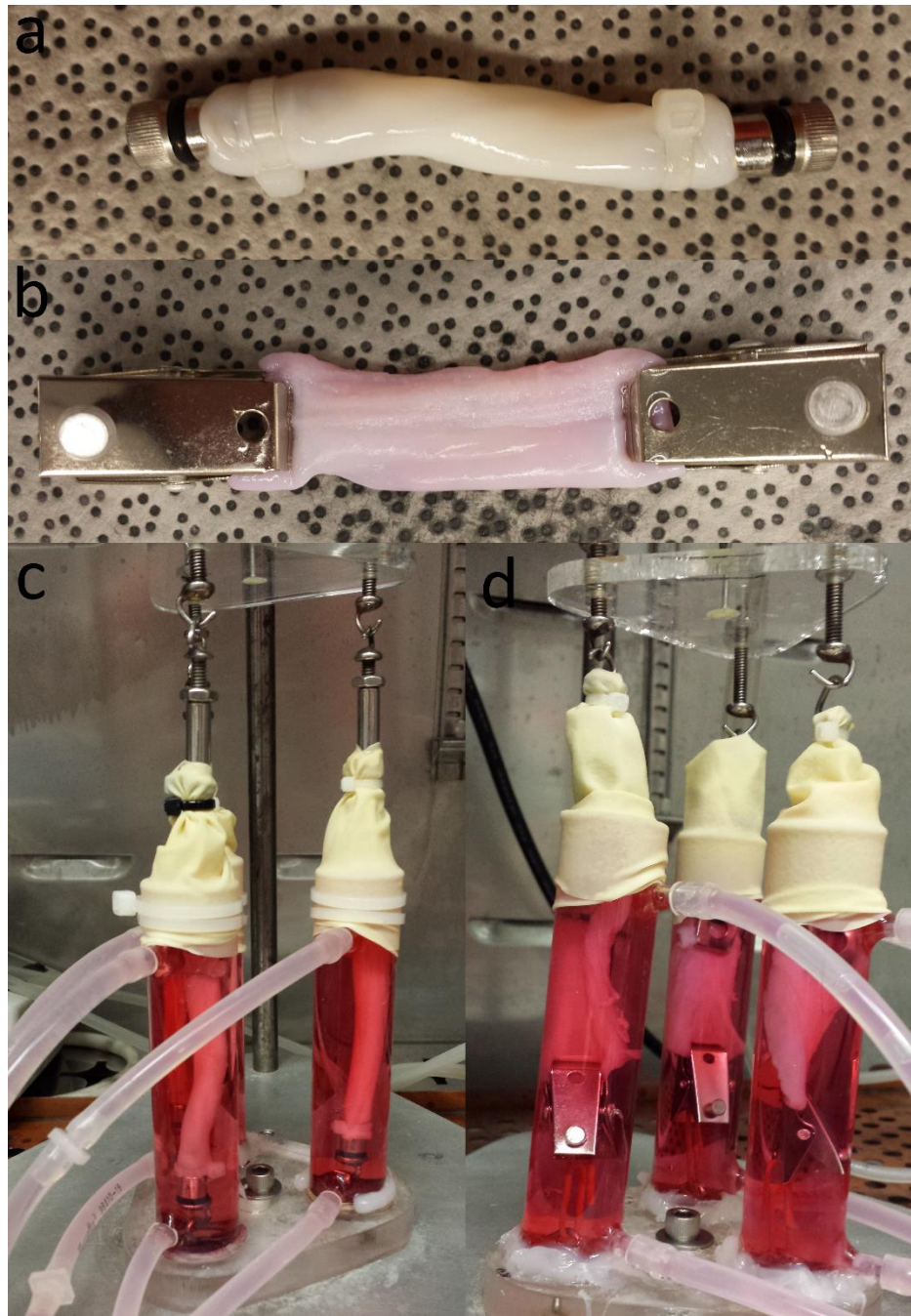
Figure 6.2: (a) Cylindrical, closed configuration of HUV for initial bioreactor culture. (b) Open flat configuration of the HUV for extended culturing. (c) Bioreactor culture of the cylindrical constructs. (d) Bioreactor culture of the flat constructs.
