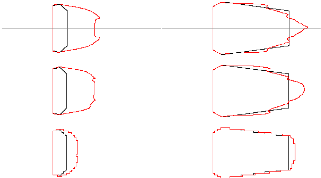
Figure 31: Burn areas at t=1800 seconds for idealized uncoupled (black) and coupled (red) simulations for initial surface winds of 3 \text{ ms}^{-1} (left) and 12 \text{ ms}^{-1} (right) and DEVS-FIRE grid resolutions of 10 m (top), 30 m (middle, and 90 m (bottom). Thin lines denote east-west lines of symmetry, and the images are zoomed to the burn areas.
