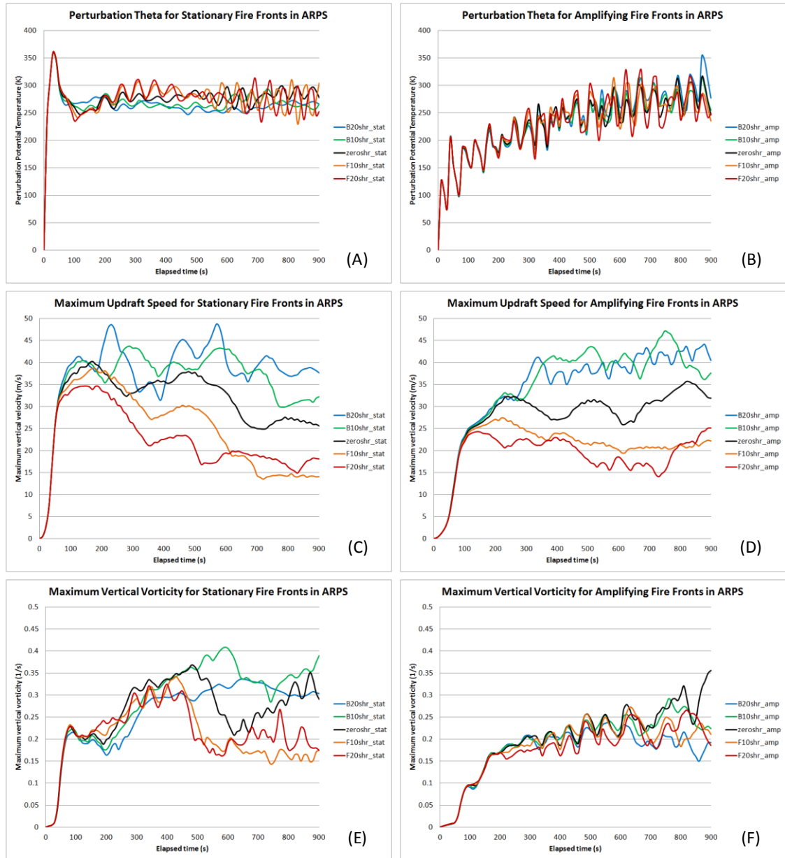
Figure 27: Maximum perturbation potential temperature, vertical velocity, and vertical vorticity for stationary (a,c,e) and amplifying fire fronts (b, d, f). Ambient vertical shear in the lowest 5 km varies by simulation: backward at 20 \text{ m s}^{-1} (blue), backward at 10 \text{ m s}^{-1} (green), no shear (black), forward at 10 \text{ m s}^{-1} (orange), and forward at 20 \text{ m s}^{-1} (red).
