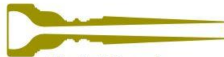
Standard Trumpet Mouthpiece: Cross-section of a standard Bach trumpet mouthpiece, based on the original design created by master trumpet artist-engineer Vincent Bach.
