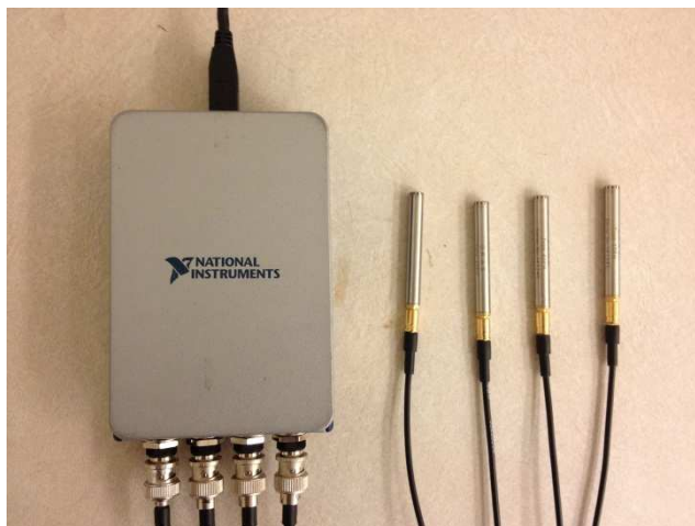
Figure 4.26: An NI cDAQ 9171 USB chassis and four microphones.
