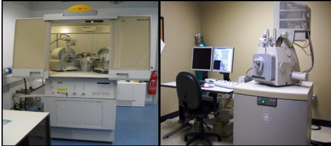
Fig. 27 (a) X-ray diffractometer, and (b) Scanning electron microscope for phase and microstructural characterization.
