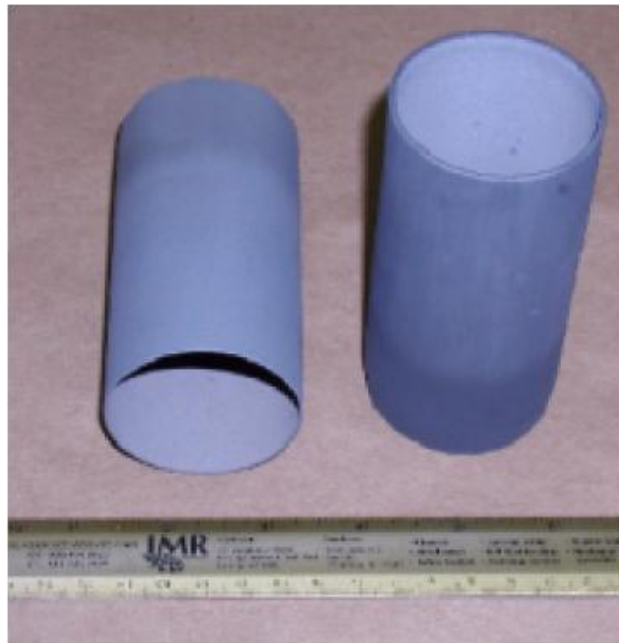
Fig. 13 TaC cylinders (50 mm in diameter, 100 mm in height, and 1.5 mm in thickness) deposited by vacuum plasma spray technique [60].
