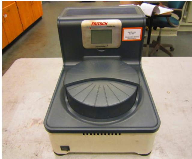
Fig. 23 High energy ball mill used for mixing powders in the OSU laboratory.
