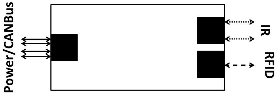
Figure IV-XXV: Weapon Block Diagram - Level 0
