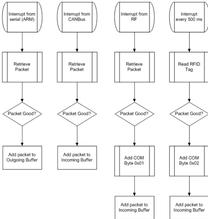
Figure IV-XIII: HIU Firmware Flowchart - Interrupts
