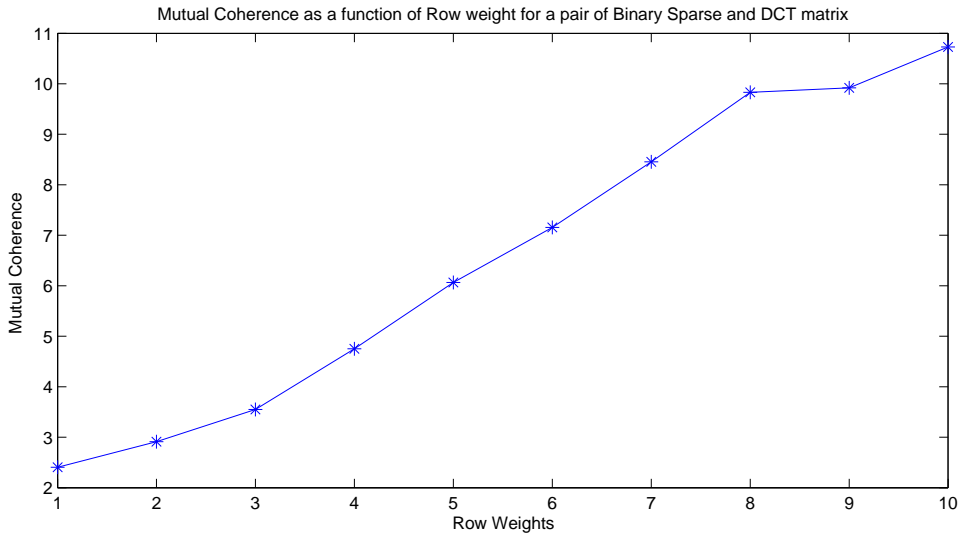
Figure 3.3: Mutual coherence vs row weight of the measurement matrix
