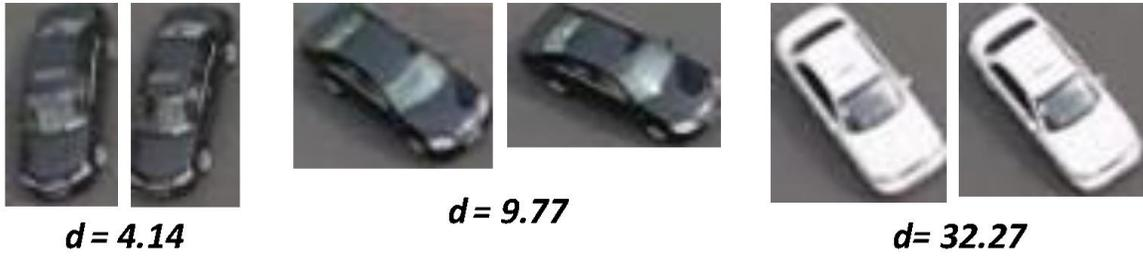
Figure 5.7: Overall similarity measure  $d$  for matched vehicles in  $I_t$  and  $I_{t+1}$
