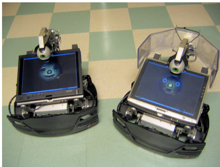
Figure 3.3: The two major hardware components of this framework – the Evolution Robotics Scorpion Robot and a Tablet PC.
