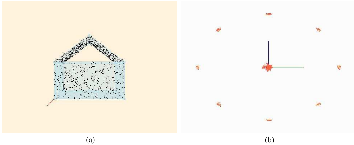
Figure 2.3: Point cloud of a simple house consisting of planes: (a) The house is made up of four walls, a floor and a roof; (b) shows the results of normal vector estimation for this point cloud. The clusters have noise from the noise in the point cloud. There are five orientations of planes which leads to ten total clusters. The solution consists of several small cluster pairs that fit tightly on the points.
