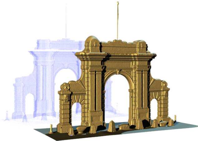
Figure 1.1: This is a surface reconstruction of a gate using LiDAR data. The point cloud is behind the reconstructed surface of the gate. This image is from www.farfieldtechnology.com .
