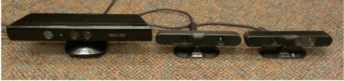
Figure 8: Left: Microsoft Kinect. Center: Asus Xtion Pro. Right: Asus Xtion Pro Live
