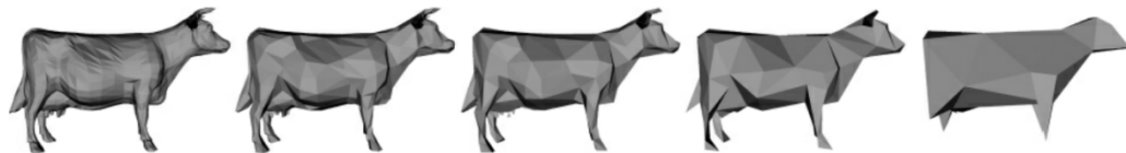
Figure 4: Mesh optimization of a model from 5,804 to 994, 532, 248, and 64 faces respectively using the quadric mesh optimization method [31]
