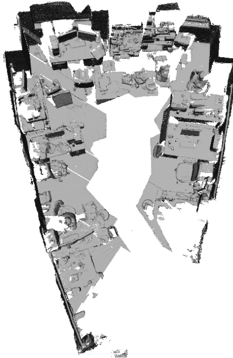
Figure 31: An example of drift occurring during a scan in a rectangular room.
