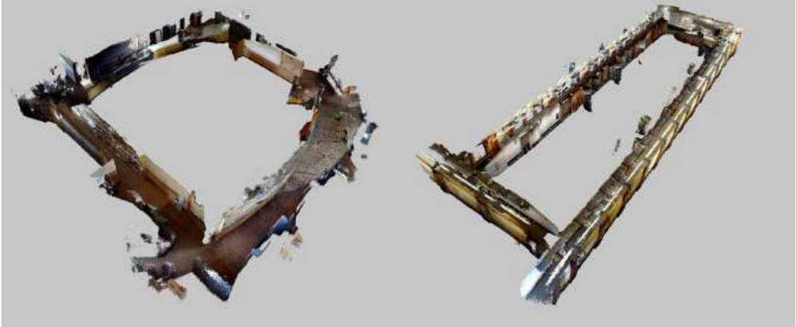
Figure 2: Dense point clouds created with RGB-D Mapping [4].
