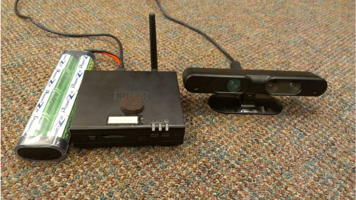
Figure 10: The Fit PC2i with a battery and an Asus Xtion Pro Live.
