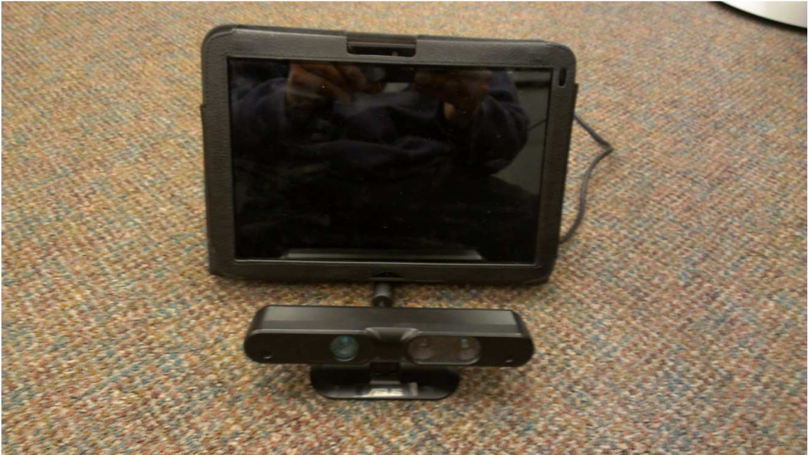
Figure 12: A Motorola Xoom with an Asus Xtion Pro Live.
