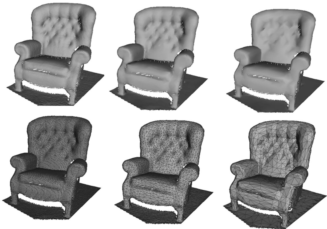
Figure 21: A chair at 3 levels of optimization. From left to right, each contains 42k, 10.6k and 7.4k triangles. The Top shows a smoothed mesh. The bottom shows a wireframe rendering.
