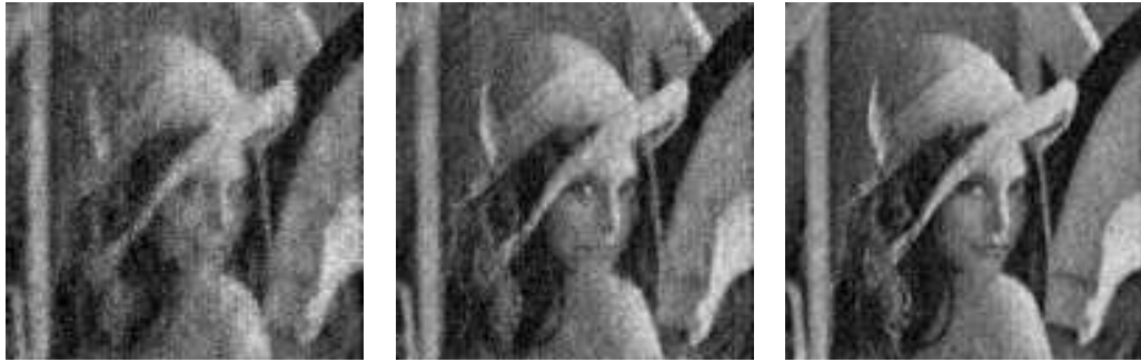
(d) Lena image reconstructed with sparse \Phi for M = 4000 . (e) Lena image reconstructed with sparse \Phi for M = 6000 . (f) Lena image reconstructed with sparse \Phi for M = 8000 .
