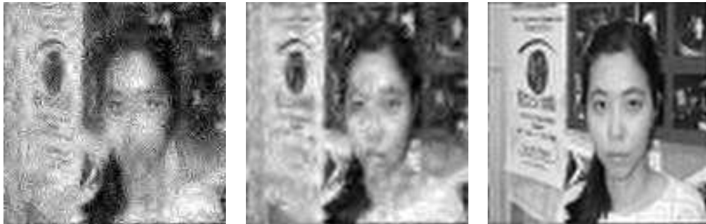
(a) Image reconstruction employing EEP- \Phi . (b) Image reconstruction employing TSWCS. (c) Image reconstruction employing UEP- \Phi .
