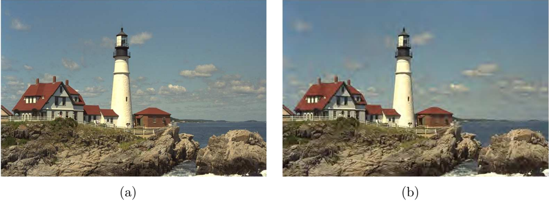
Figure 3.13: An example of a reference image and highly distorted version from the LIVE database are shown. The distortion image contains JPEG2000 artifacts.
