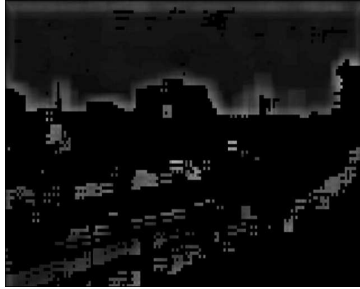
Figure 3.7: The two maps are multiplied together. The resultant map shows the LMSE of only visible patches in the image. This map is collapsed using the vector two norm of equation (3.8).
