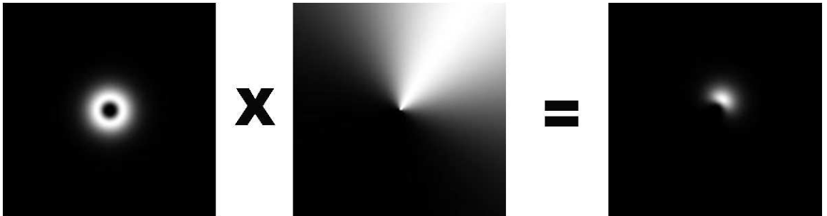
Figure 3.8: Three images are shown of a single log-Gabor filter. The first is the frequency scaling operation defined by equation (3.9) and the second is the orientation defined by equation (3.10). The last is the multiplication of the filters defined by equation (3.11). All pictures are magnitudes in the frequency domain.
