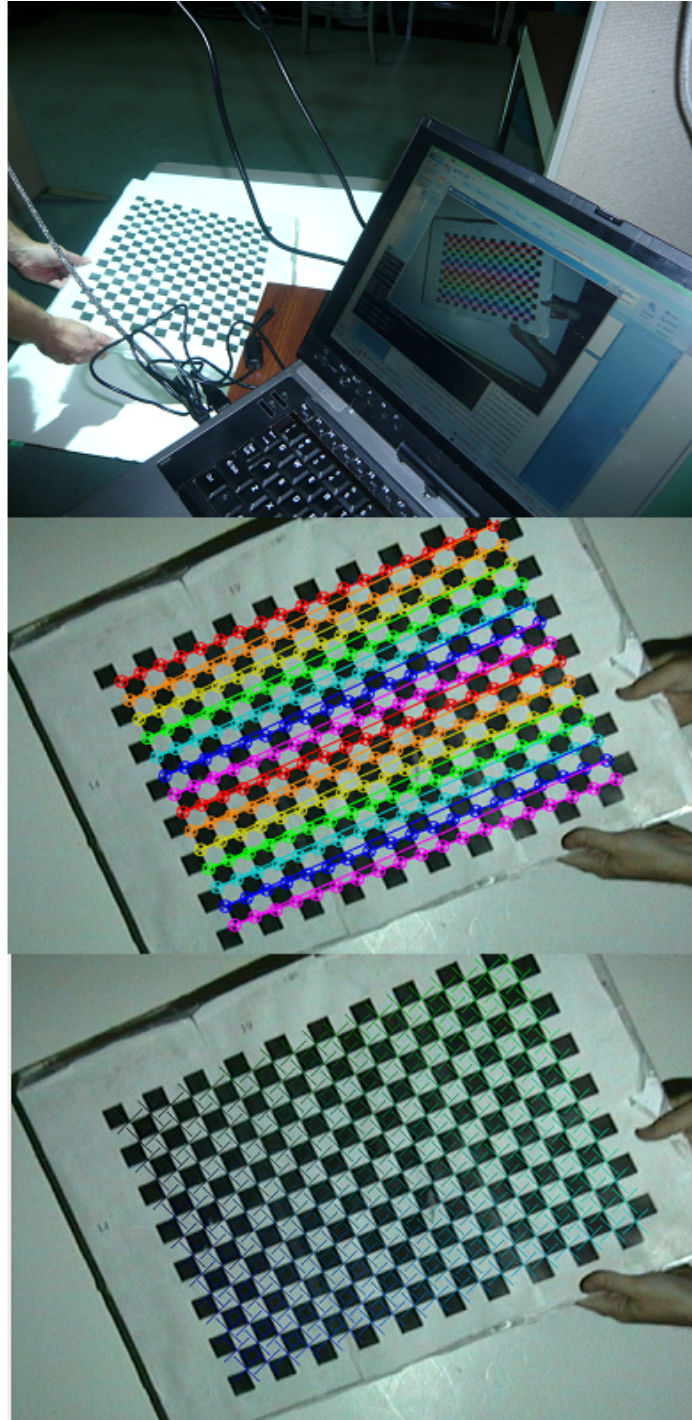
Figure 5: Top: Camera undergoing calibration with a physical calibration pattern. Middle: Physical pattern with found corners. Bottom: Reconstructed corners using 3D points and calibration information.
