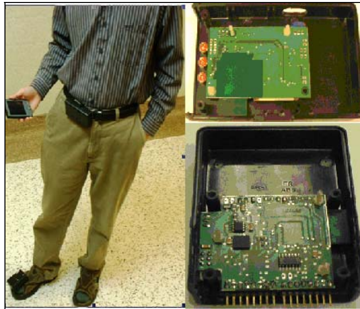
Figure 1: Prototypes of Wearable Position Tracking System (left) and Data Processing Unit (right) Inertial Sensor unit (Bottom Right)
