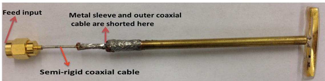
Figure 7.3: Antenna C including dielectric substrate and acrylic connected to the feed network
