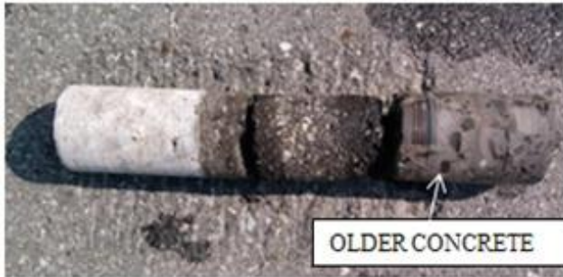
Figure 2.4 – A typical core from an Oklahoma whitetopping.
