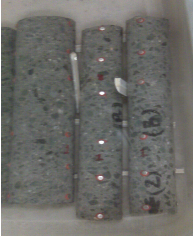
Fig. 3.6. General demec layout for one line.
