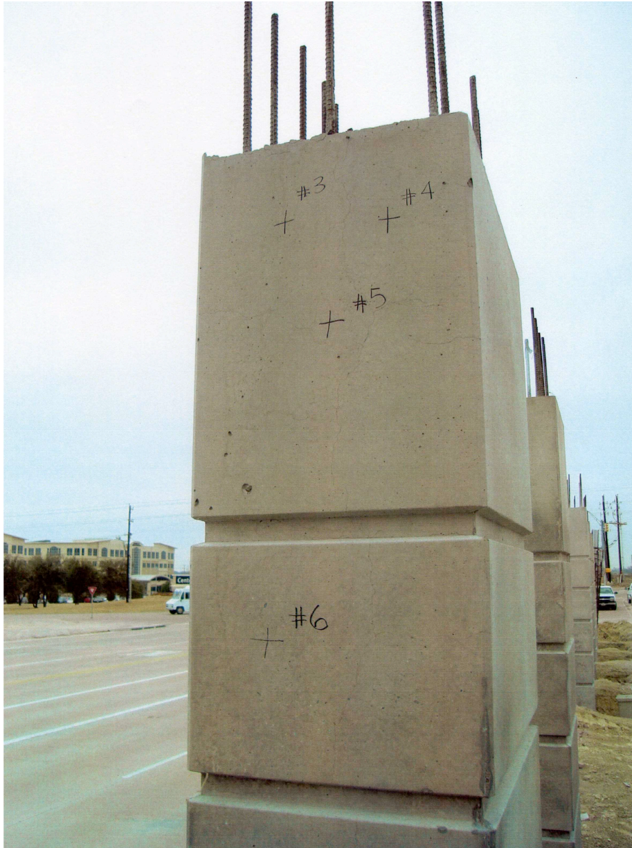
Fig. 3.2. Column cored for the Texas cores (McMillan, 2009).
