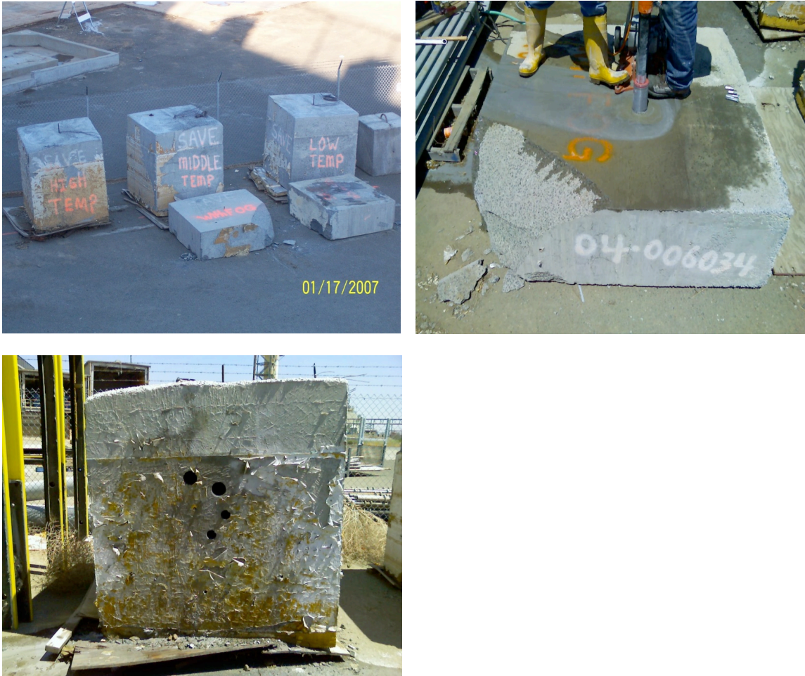
Fig. 3.5. Information only cast-in-place blocks for coring and temperature recording.
