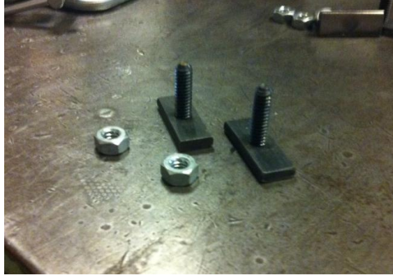
Figure 3.2 Tabs and Nuts for STS-II Assembly
