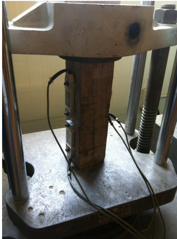
Figure 3.6 Testing the STS-II and Sensors in a Compression Machine
