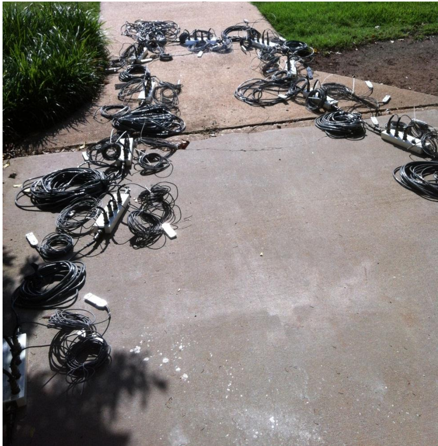
Figure 3.7 Testing All (40) Strain Sensors
