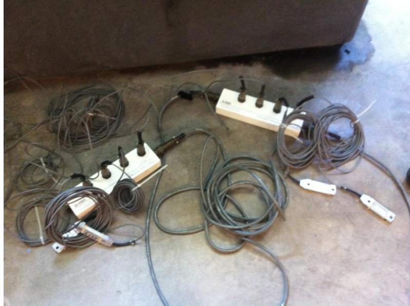
Figure 3.4 STS-II Boxes and Wires
