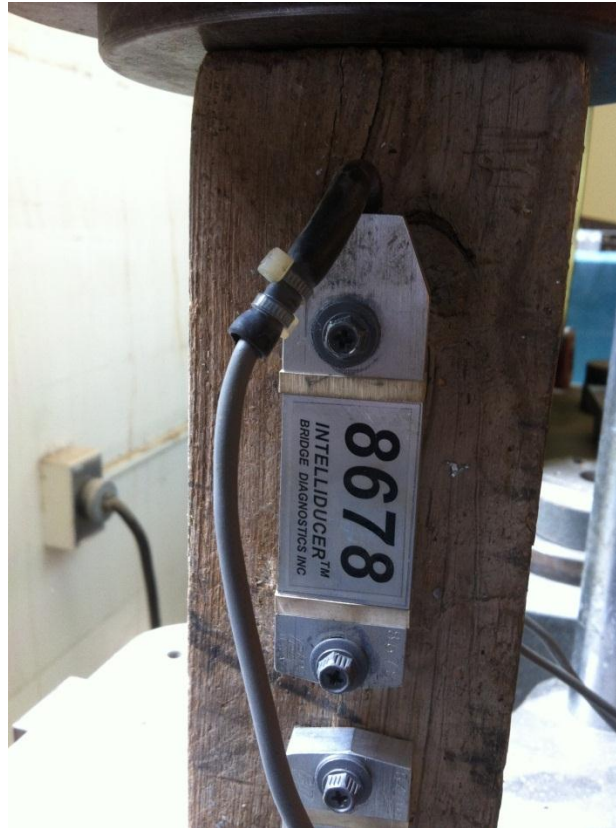
Figure 3.1 STS-II Strain Transducer Installed in 4X4
