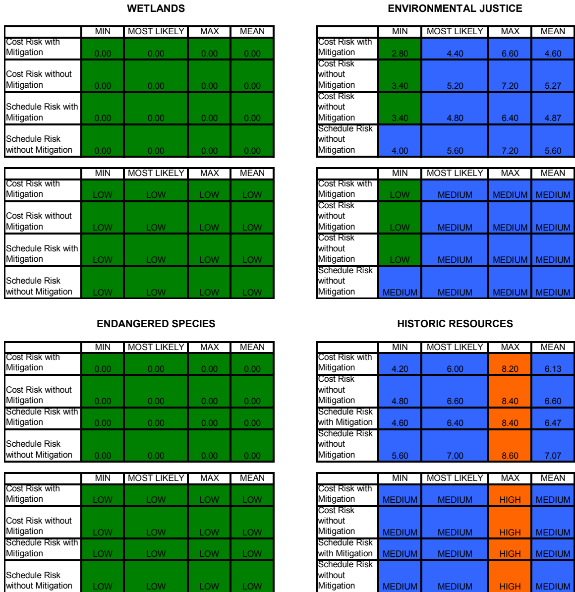
Figure 44. Results of fuzzy simulations for the City of South San Francisco, light railway mode. Results from individual matrices: wetlands, environmental justice, endangered species, and historic resources.
