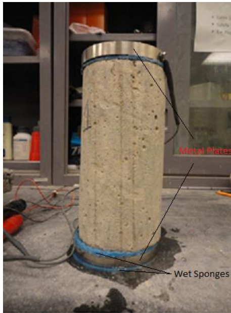
Figure 8: Measuring resistivity of concrete by two-plate resistivity method
