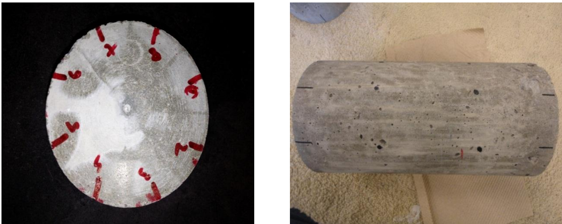
Figure 10a&b: Cylinder with spots marked at the places where resistivity is measured.
