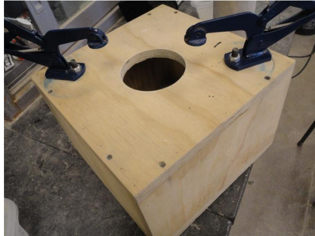
Figure 3: Wooden box with anchors fixed to it for testing concrete cylinders
