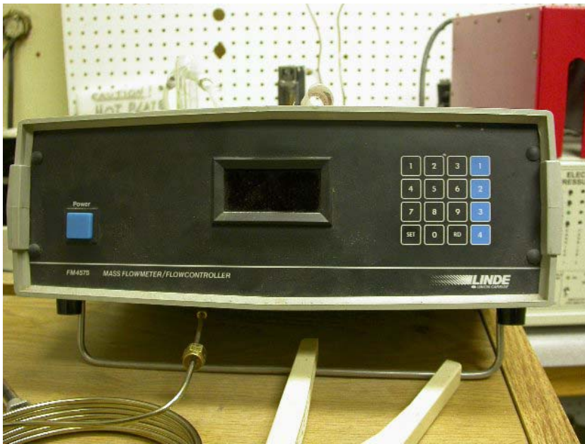
Figure 16: Mass Flow Controller Panel
