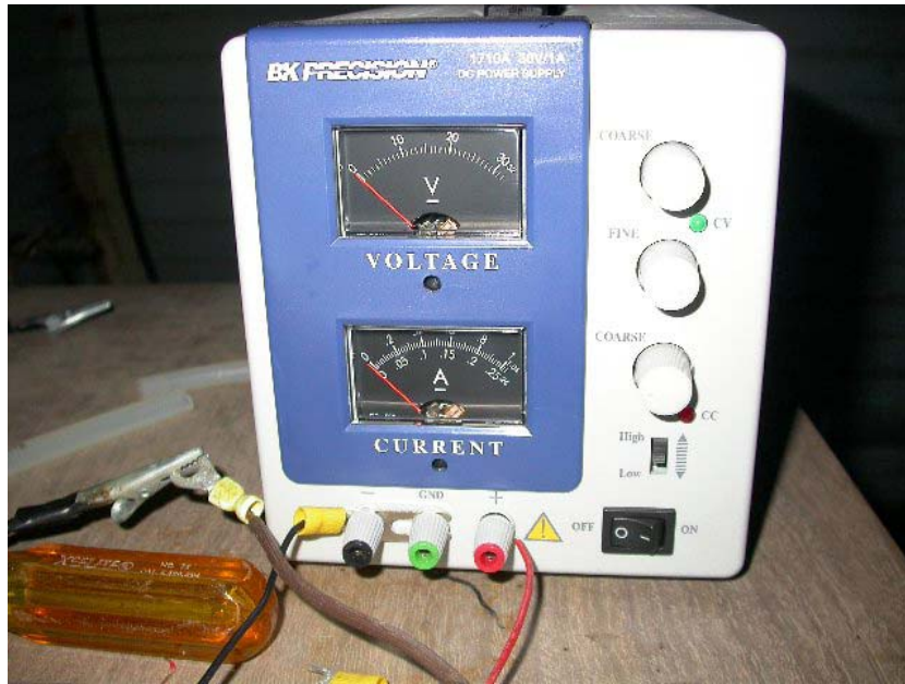
Figure 12: Secondary Power Source
