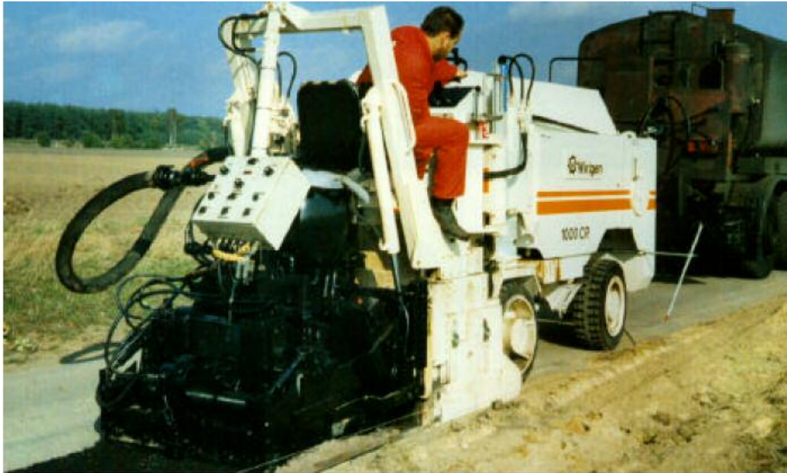
FIGURE 2-1 A Self Contained Single Unit CIR Train [10].
