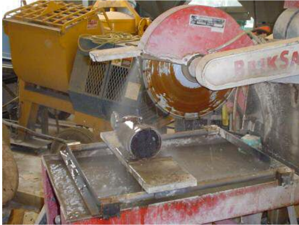
FIGURE 3-3 Sample is Sawed to Obtain Parallel Faces.
