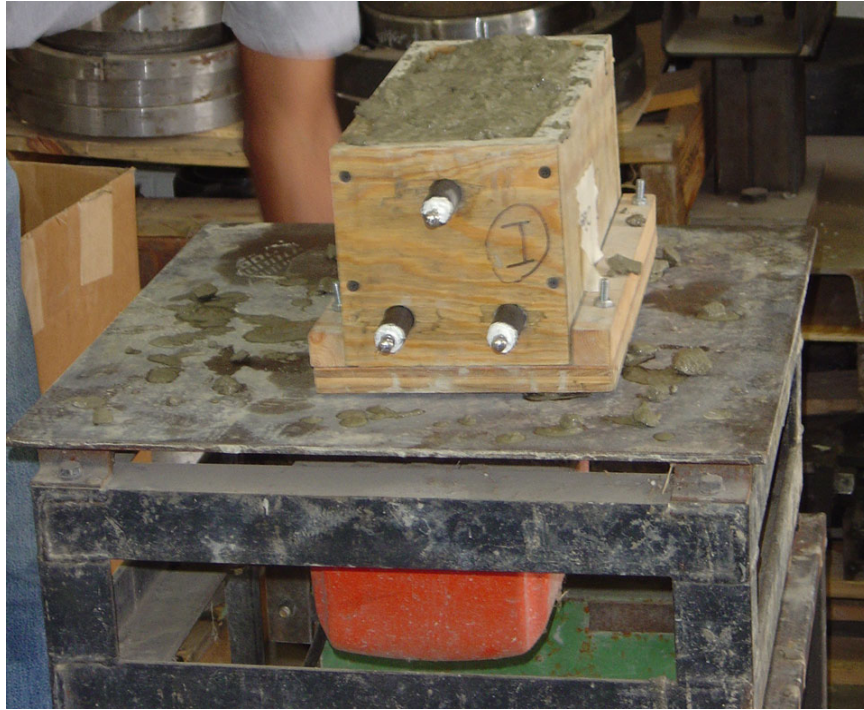
Figure 20: Consolidation of Concrete
