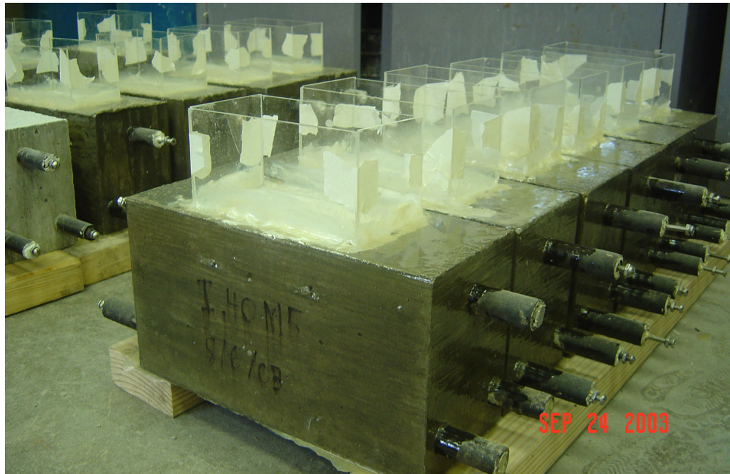
Figure 18: Completed G 109 Specimens
