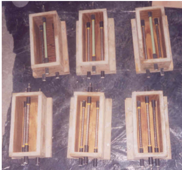
Figure 19: Completed Reinforcing Bars in Formwork
