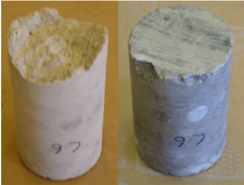
Figure 30: Core C6 Before and After Sawing End
