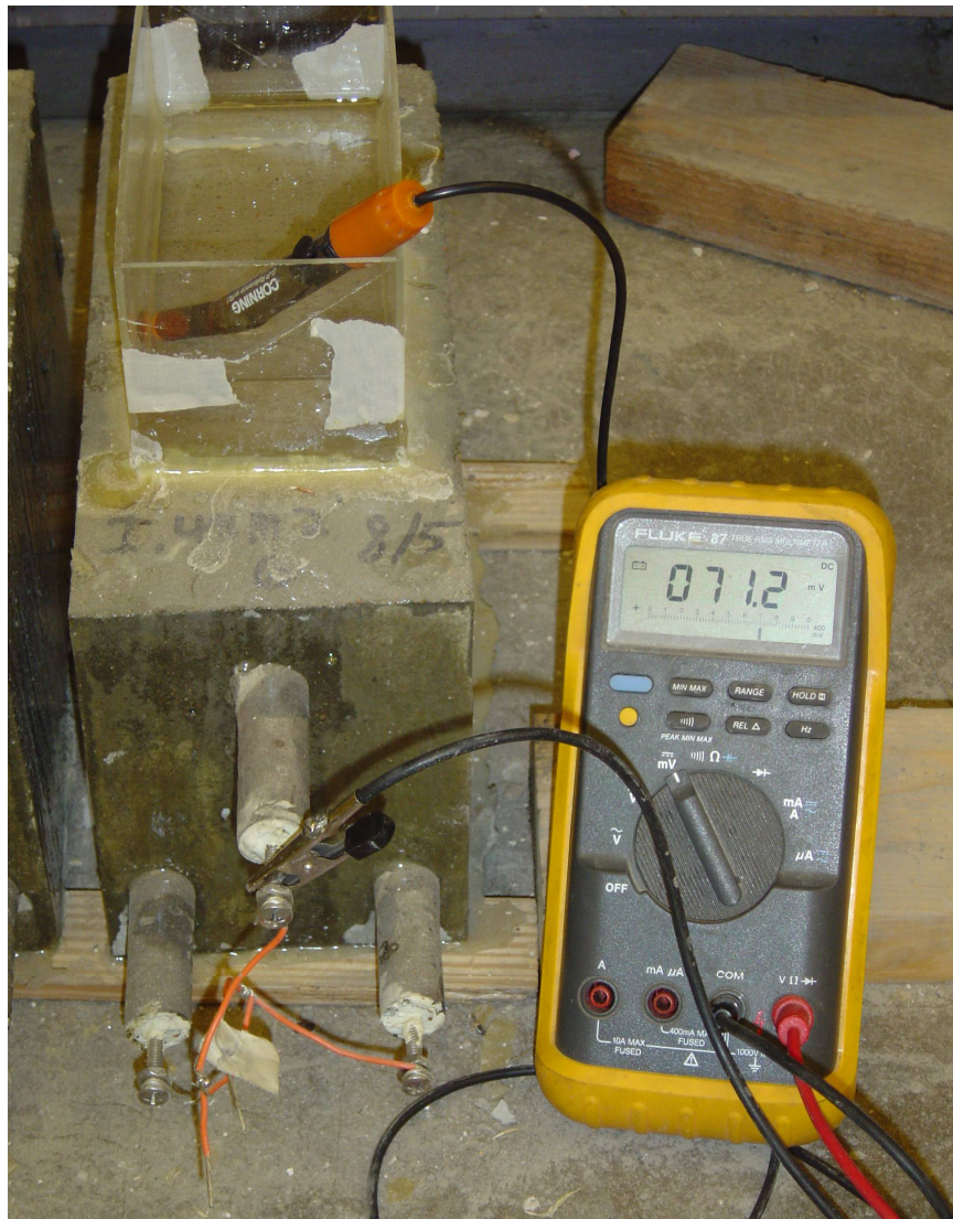
Figure 22: Measurement of Corrosion Potential
