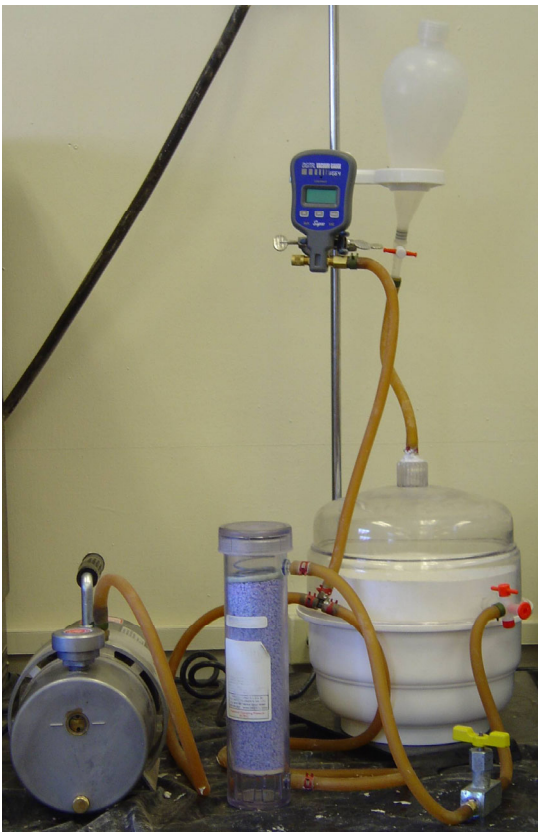
Figure 32: Vacuum Saturation Apparatus for ASTM C 1202
