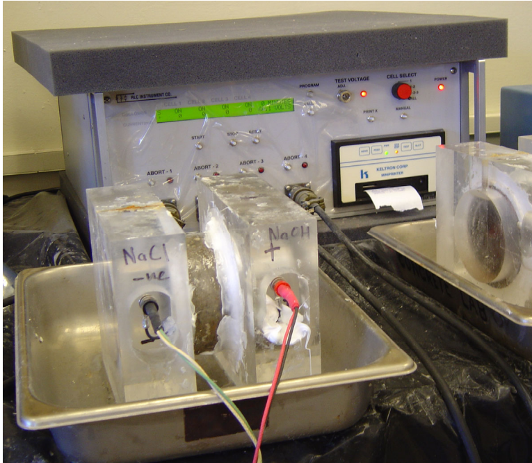
Figure 33: Applied Voltage Cell with Constant Voltage Power Supply and Data Readout Apparatus
