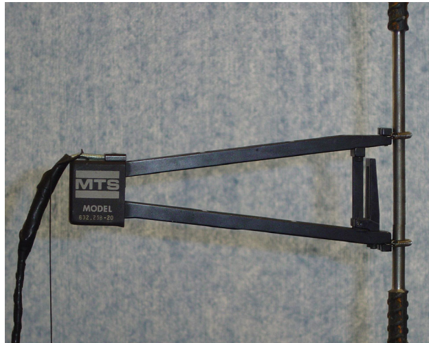
Figure 23: Attachment of Extensometer
