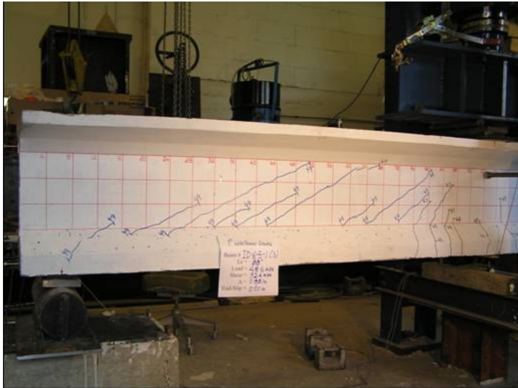
Photo of the South end of the beam ID-6-5-1 showing the first web shear cracking
