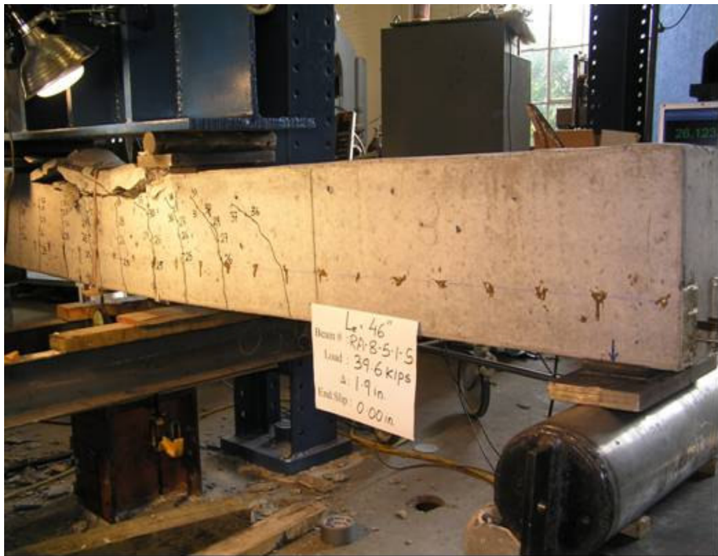
Cracking pattern at South end for Beam RA-8-5-1 (South side being tested)
