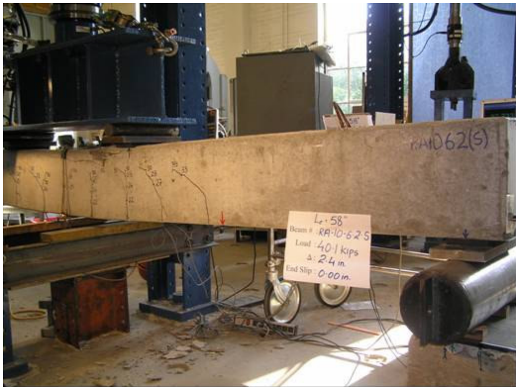
Cracking pattern for Beam RA-10-6-2 being loaded at South end
