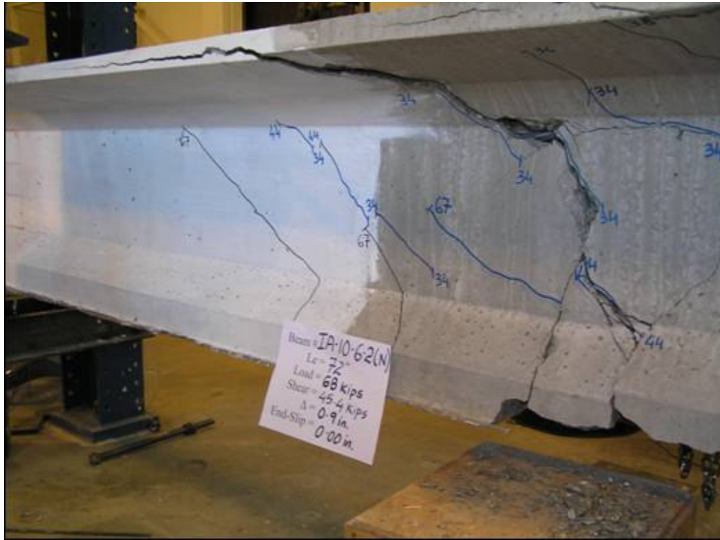
Photo of the North end of the beam IA-10-6-2 showing shear failure in the South side shear zone.
