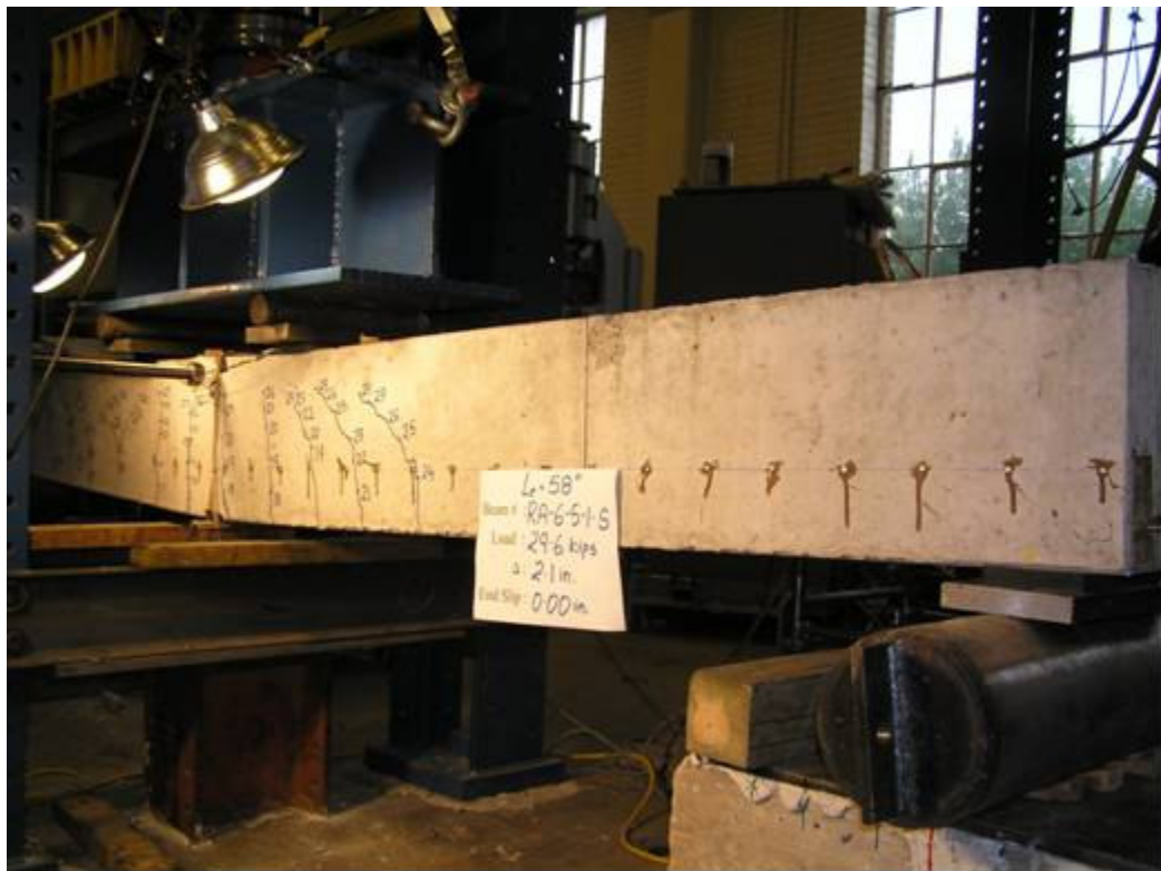
Cracking pattern for Beam RA-6-5-1 being loaded at South end
