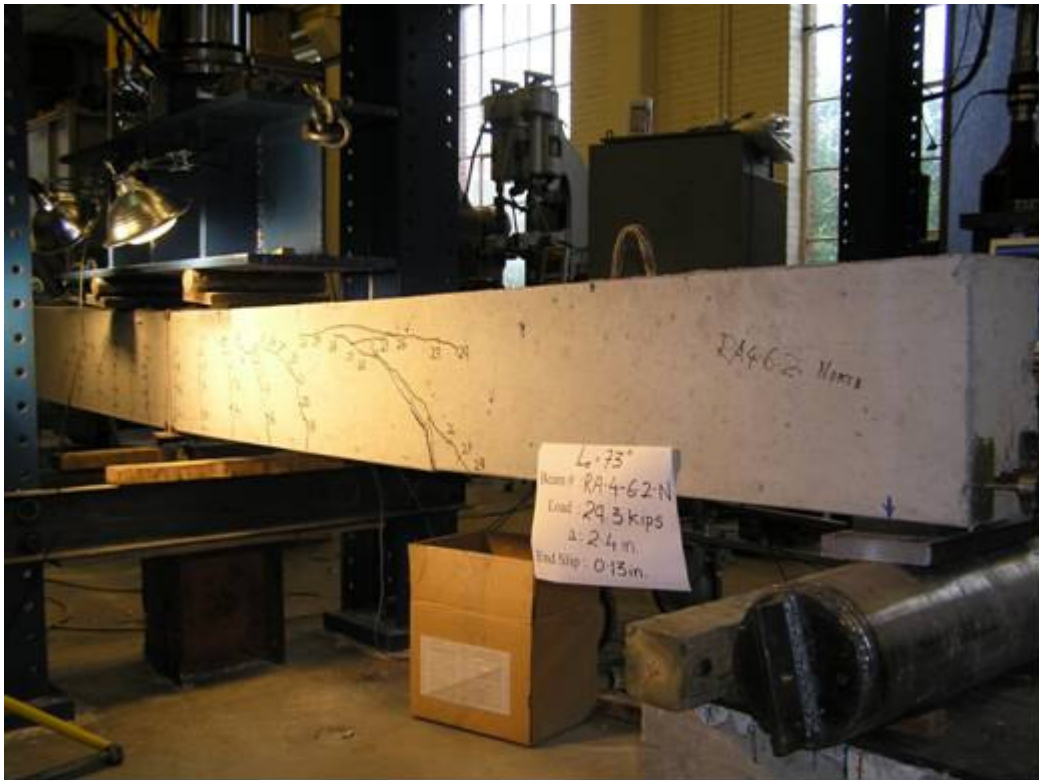
Cracking pattern for Beam RA-4-6-2 being loaded at North end
