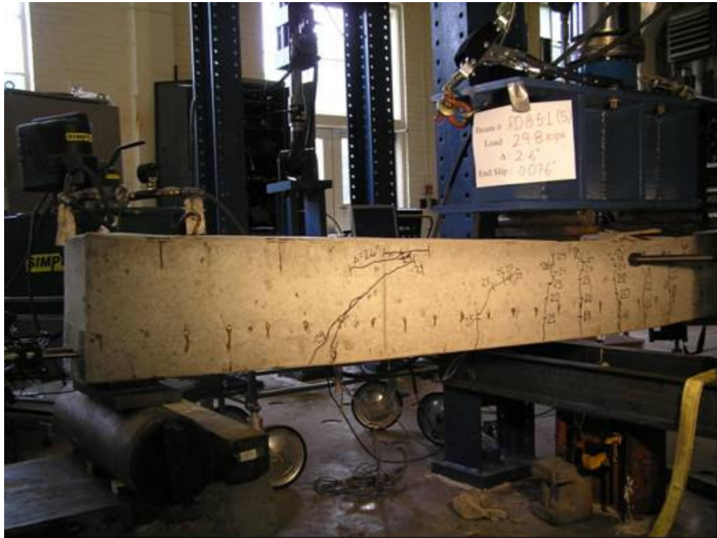
Cracking pattern for Beam RD-8-5-1 being loaded at South end
