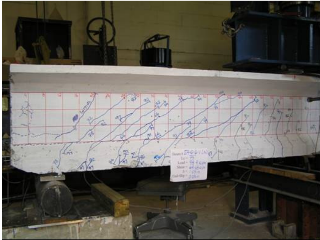
Photo of South end of beam IA-6-6-1 showing the cracking pattern at the maximum load
