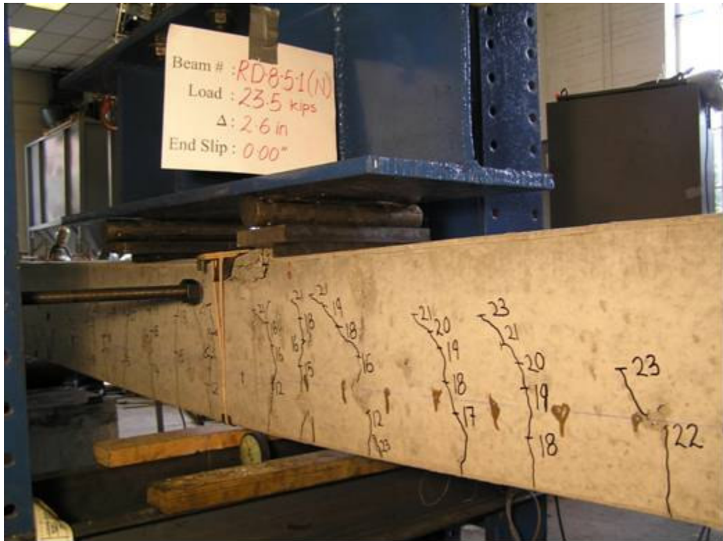
Cracking pattern for Beam RD-8-5-1 being loaded at North end
