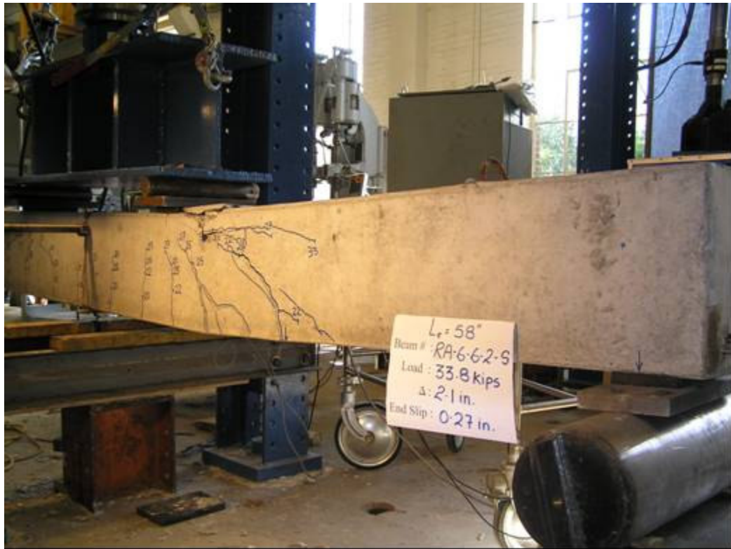
Cracking pattern for Beam RA-6-6-2 being loaded at South end
