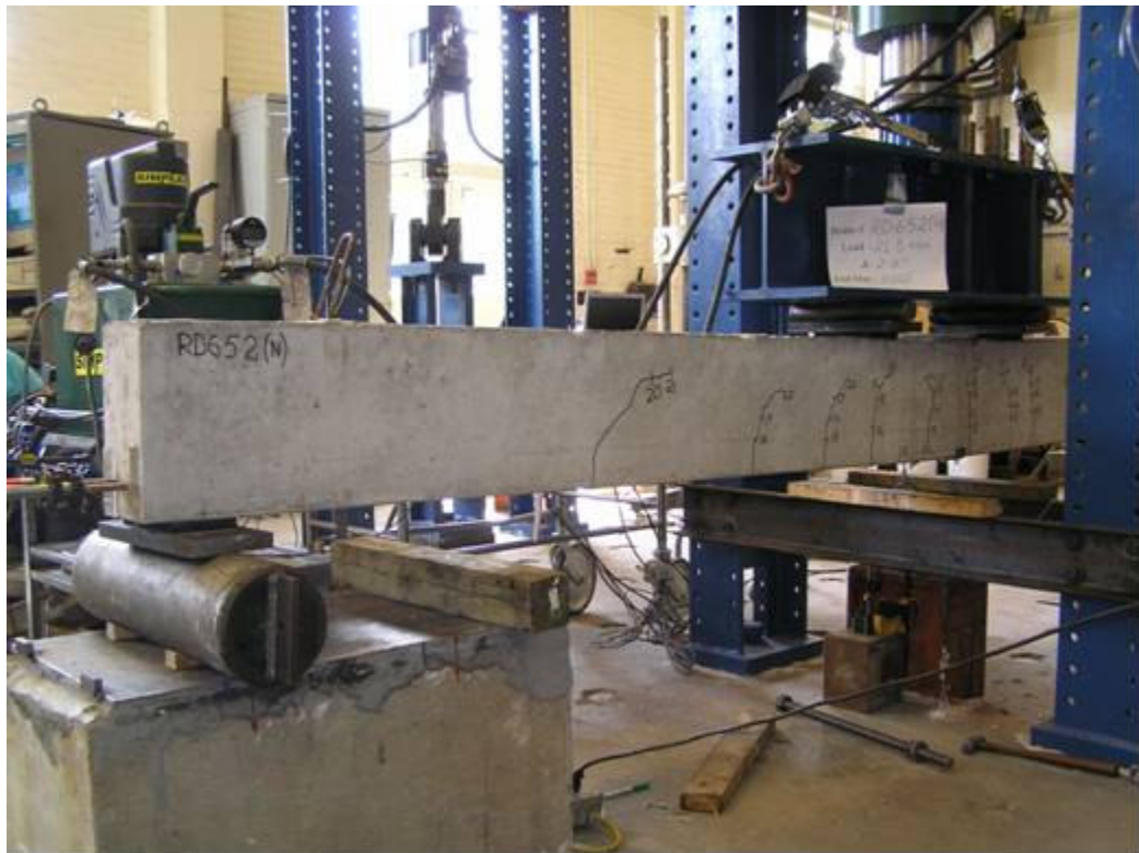
Cracking pattern for Beam RD-6-5-2 being loaded at North end.
