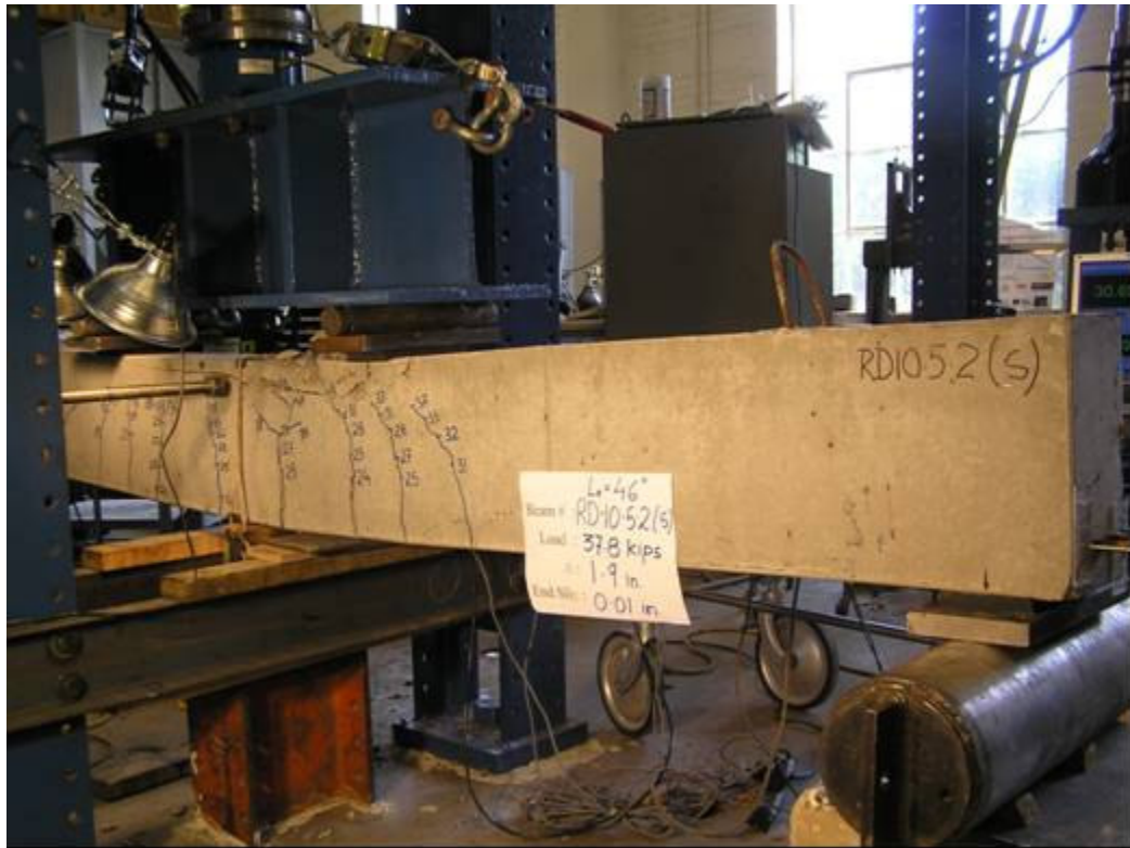
Cracking pattern for Beam RD-10-5-2 being loaded at South end
