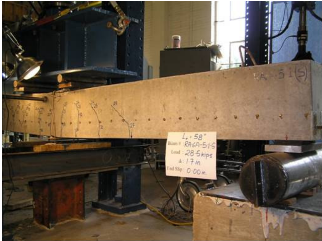
Cracking pattern for Beam RA-6A-5-1 being loaded at South end.
