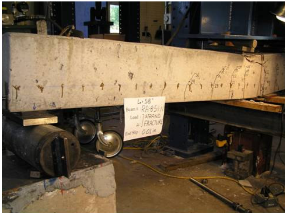
Cracking pattern for Beam RA-8-5-1 being loaded at North end
