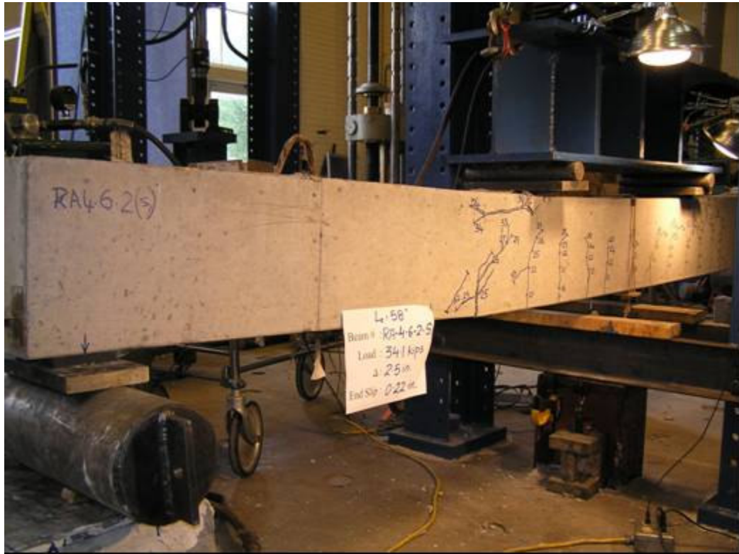
Cracking pattern for Beam RA-4-6-2 being loaded at South end
