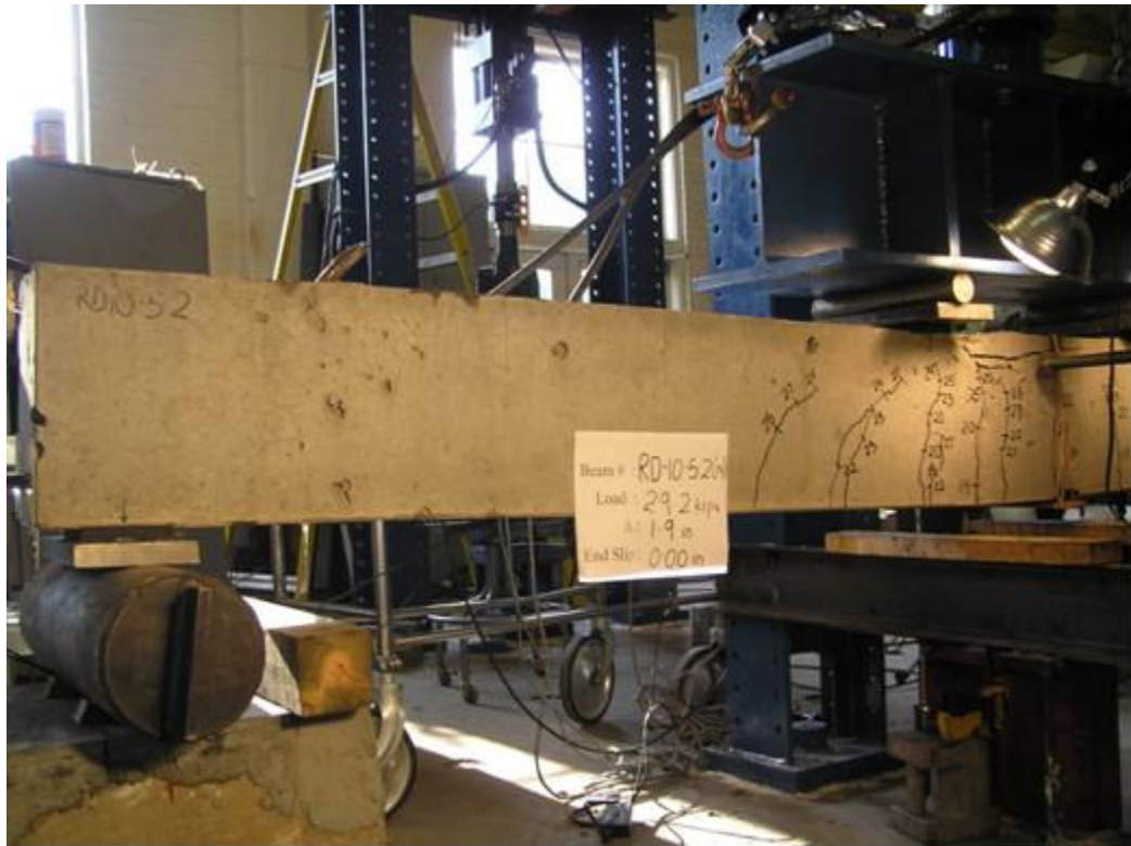
Cracking pattern for Beam RD-10-5-2 being loaded at North end
