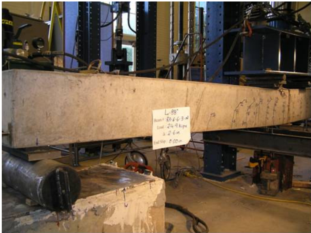
Cracking pattern for Beam RA-6-6-3 being loaded at North end
