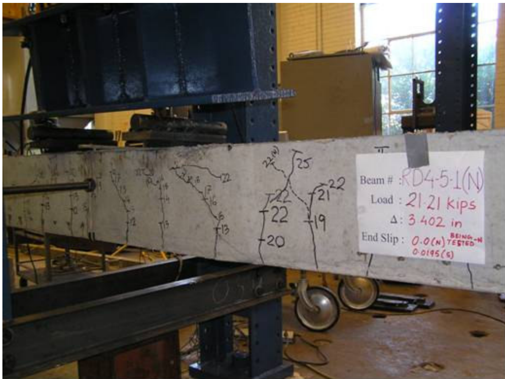
Cracking pattern for Beam RD-4-5-1 being loaded at North end.
