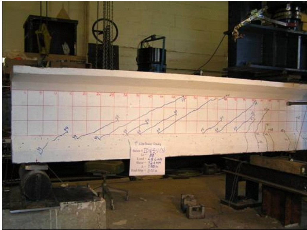
Figure 4.12: Photo of the South end of the beam ID-6-5-1 showing the first web shear cracking
