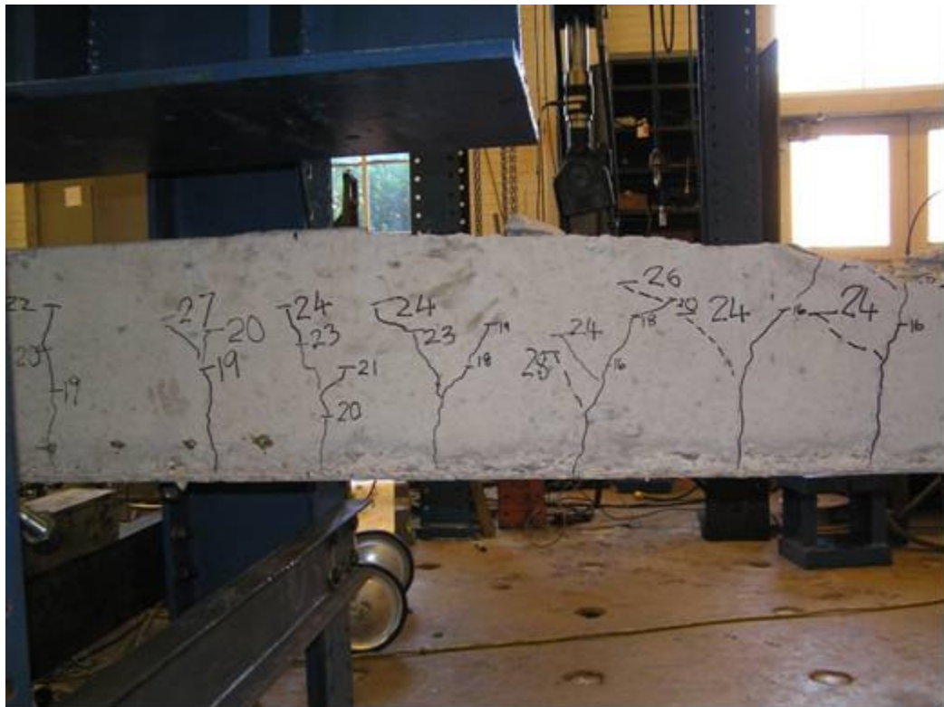
Cracking pattern for Beam RB-4-5-1 being loaded at South end
