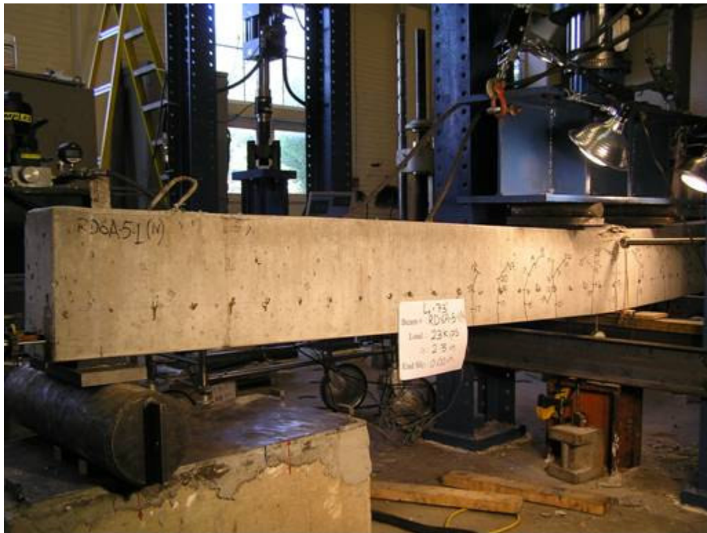
Cracking pattern for Beam RD-6A-5-1 being loaded at North end.
