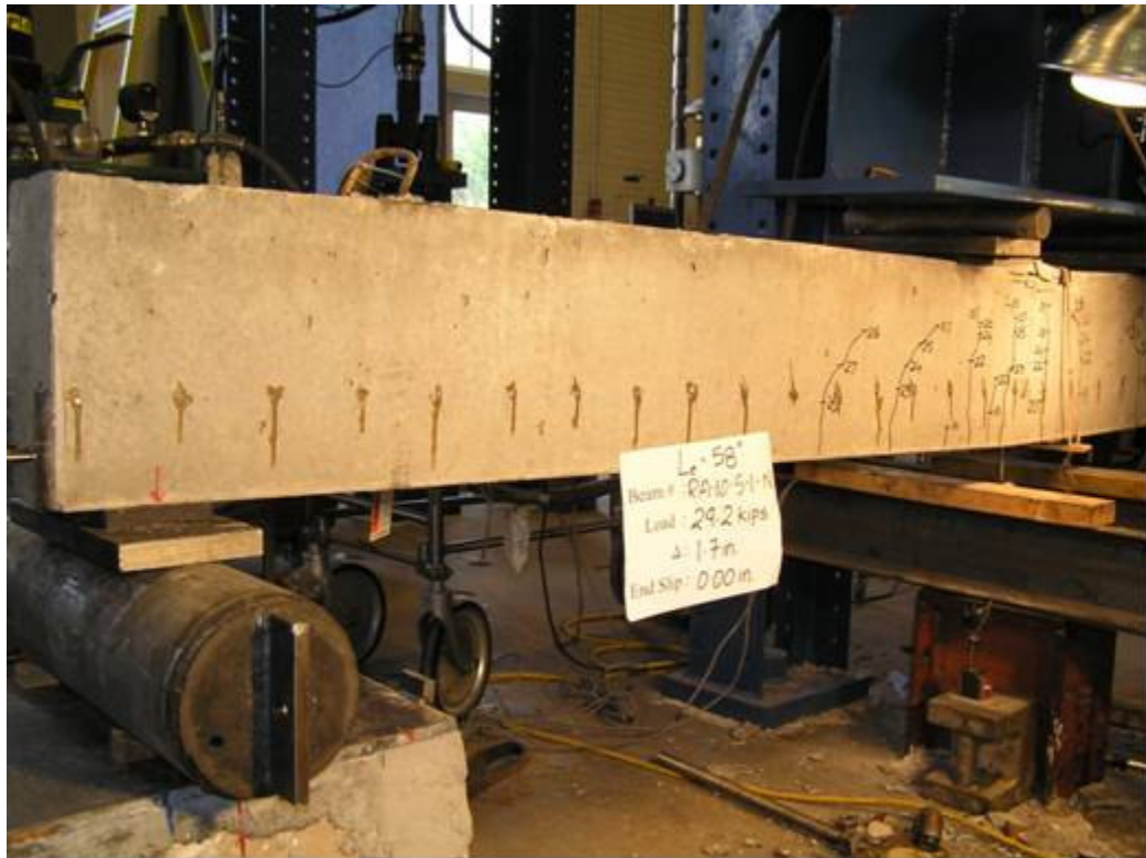
Cracking pattern for Beam RA-10-5-1 being loaded at North end
