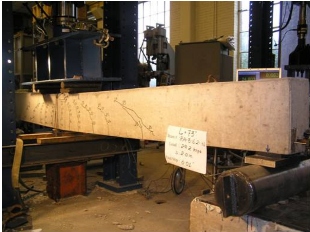
Cracking pattern for Beam RA-8-6-2 being loaded at North end
