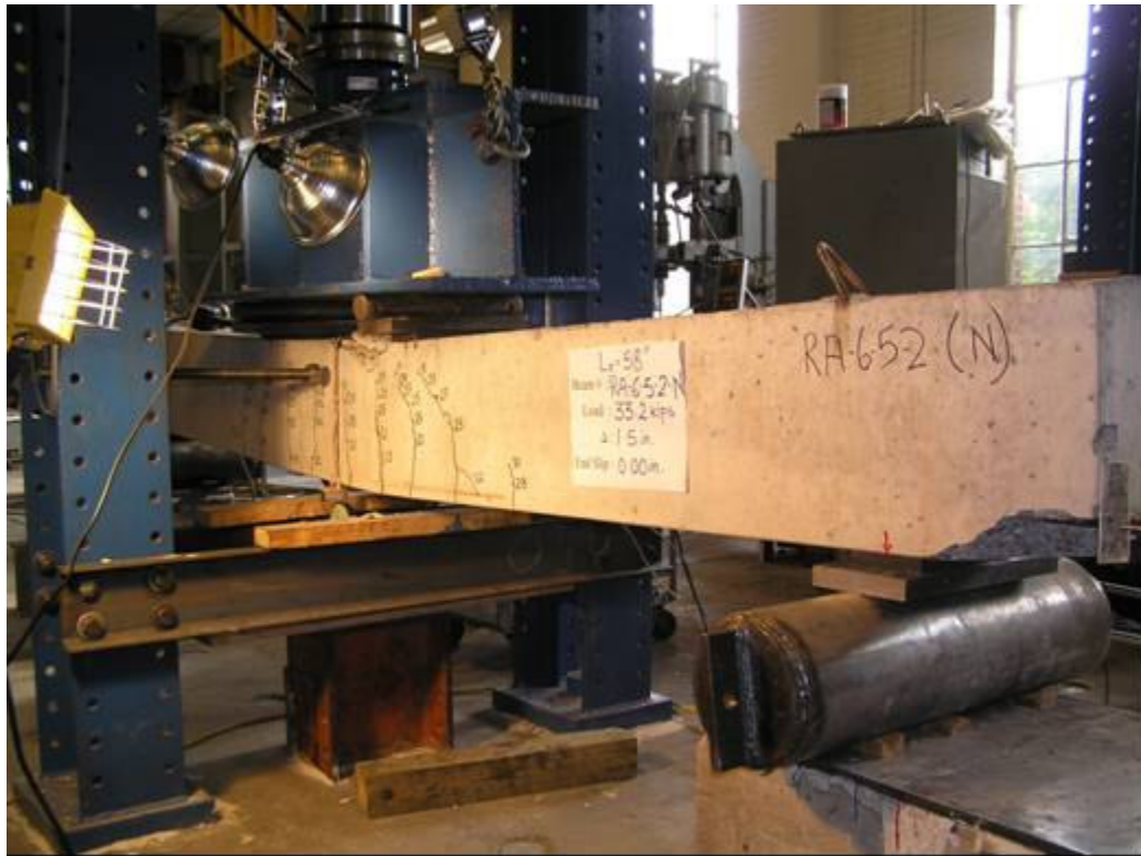
Cracking pattern for Beam RA-6-5-2 being loaded at North end
