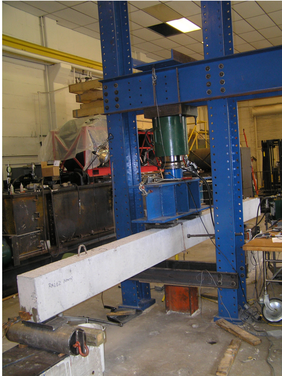
Figure 3.6: Test frame with one of the rectangular beams in place
