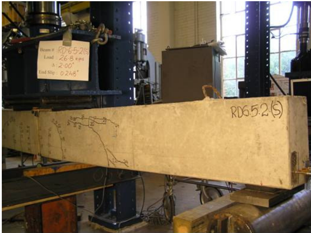
Cracking pattern for Beam RD-6-5-2 being loaded at South end.
