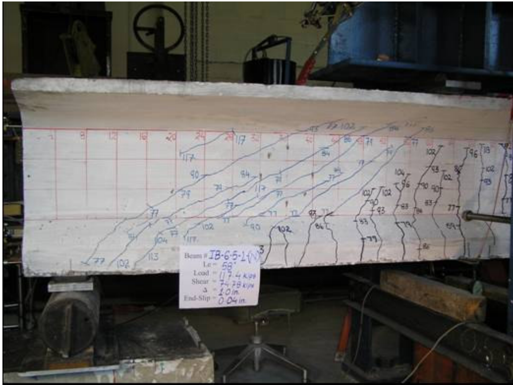
Photo of North end of beam IB-6-5-1 showing the cracking pattern at the maximum load
