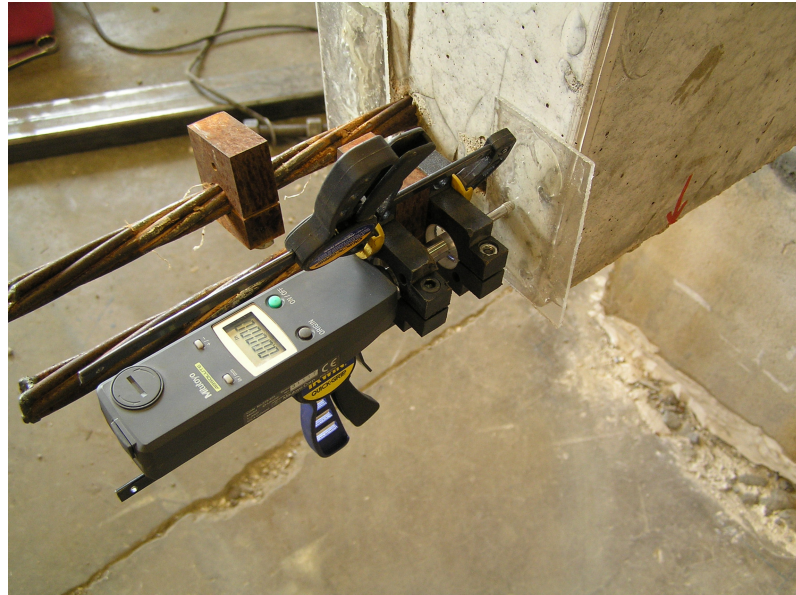
Figure 3.13: Photo showing digital dial gauge attached to the strands at the opposite end for one of the rectangular beams
