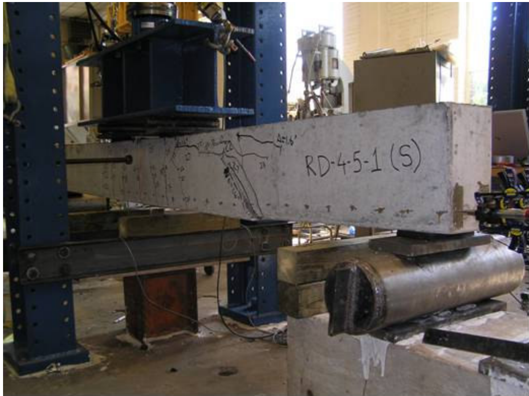
Photo Showing cracking pattern for Beam RD-45-1 being loaded at South end.
