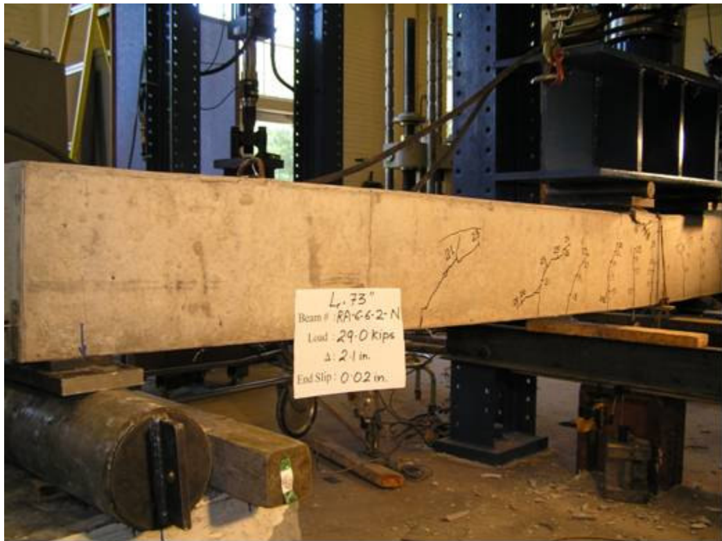
Cracking pattern for Beam RA-6-6-2 being loaded at North end
