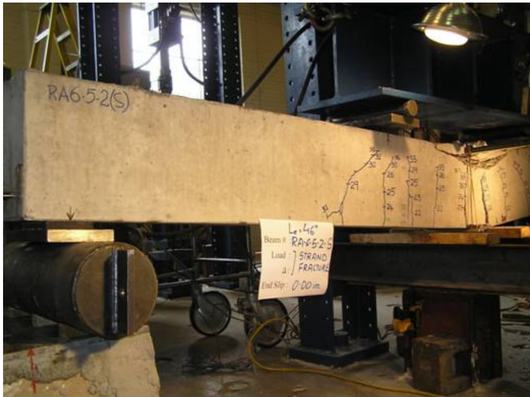
Cracking pattern for Beam RA-6-5-2 being loaded at South end
