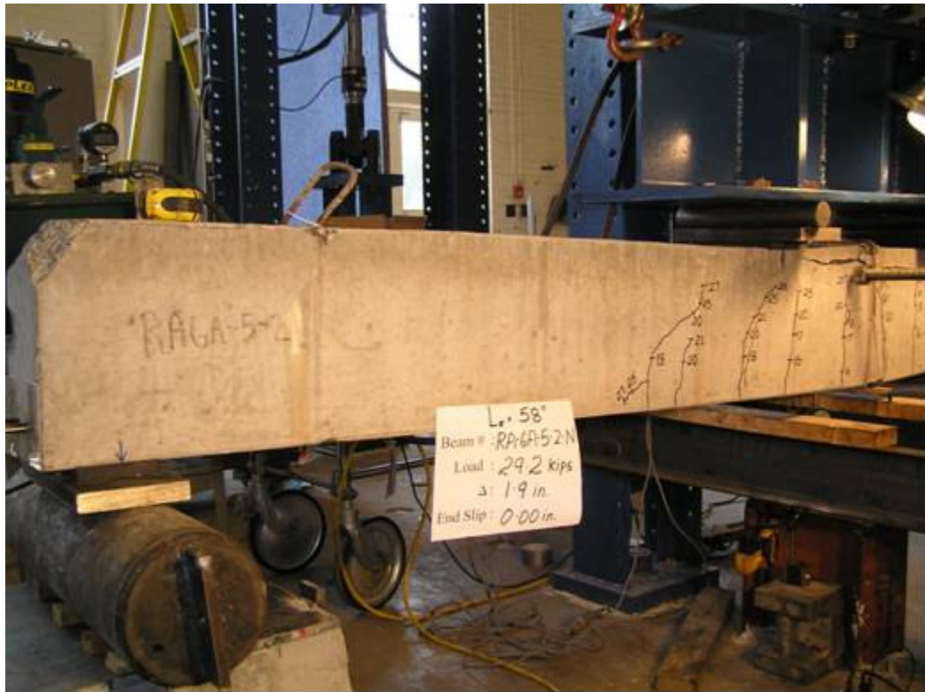
Cracking pattern for Beam RA-6A-5-2 being loaded at North end
