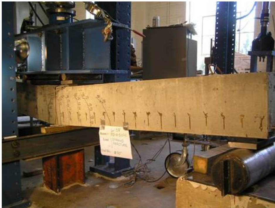
Cracking pattern for Beam RD-10-5-1 being loaded at North end
