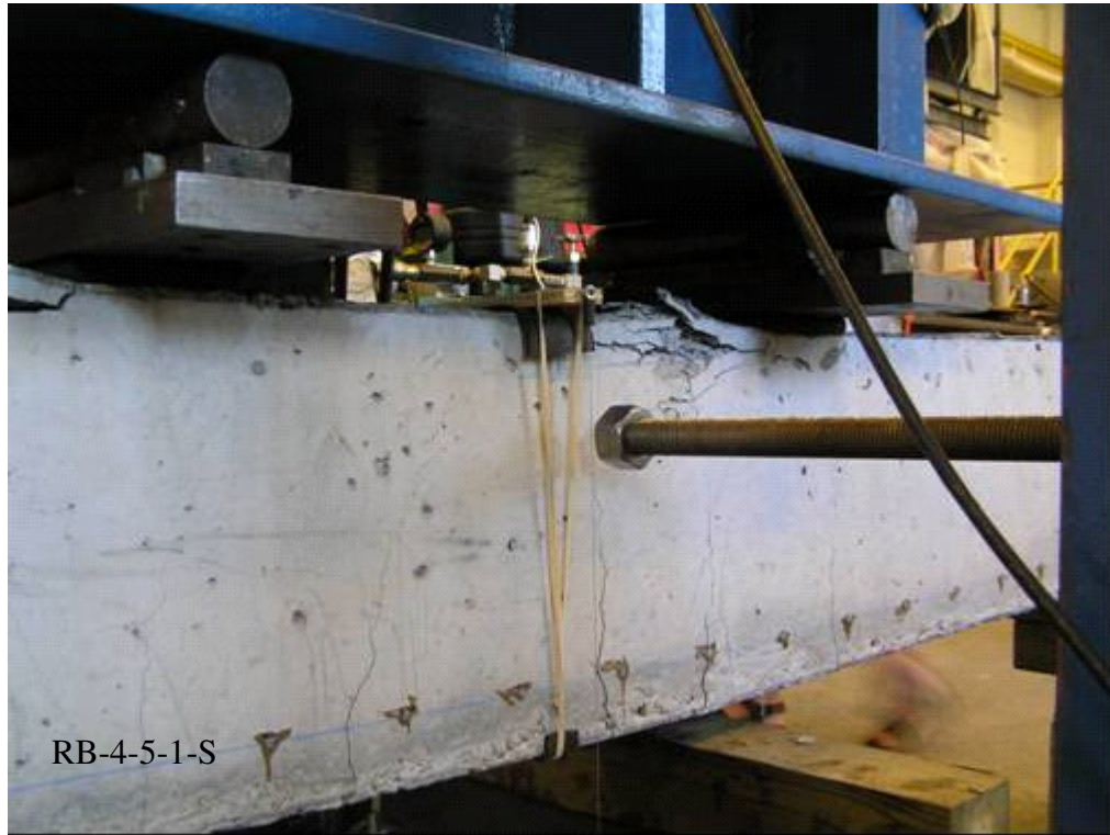
Figure 4.2: Concrete crushing at the top surface of concrete (Test – RB-4-5-1 S)
