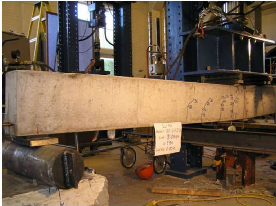
Cracking pattern for Beam RA-10-6-2 being loaded at North end
