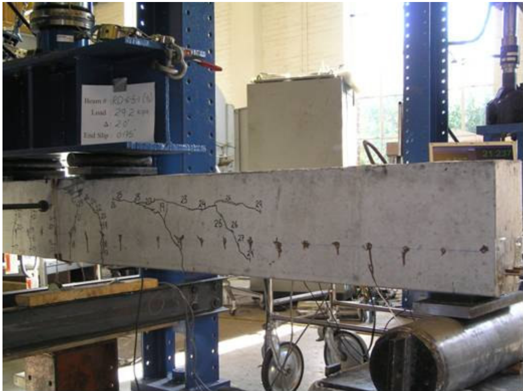
Cracking pattern for Beam RD-6-5-1 being loaded at South end.
