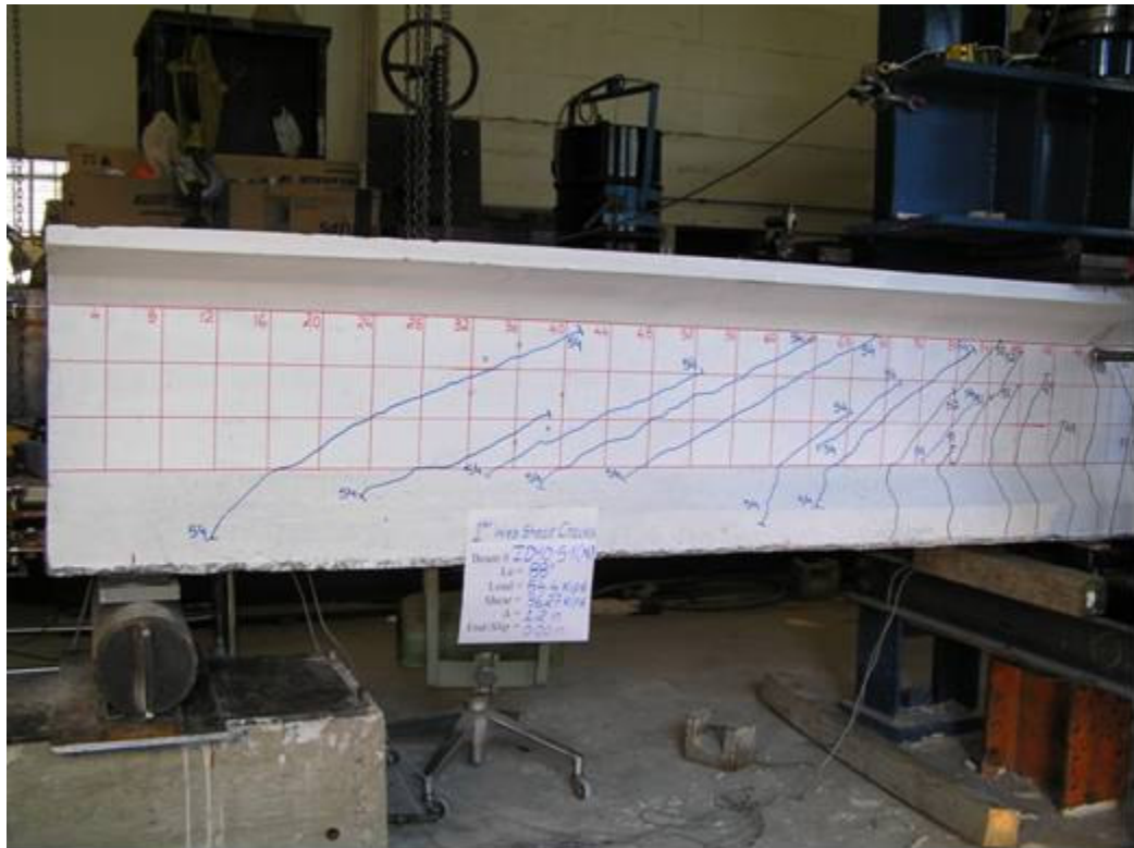
Photo of the North end of the beam ID-10-5-1 showing the first web shear cracking
