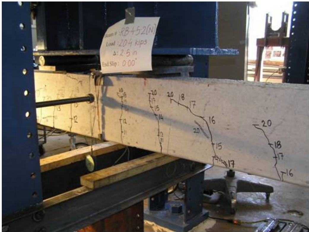
Photo showing cracking pattern for Beam RB-4-5-2 being loaded at North end
