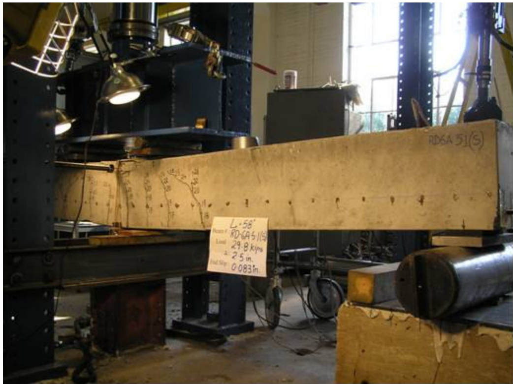
Cracking pattern for Beam RD-6A-5-1 being loaded at South end.
