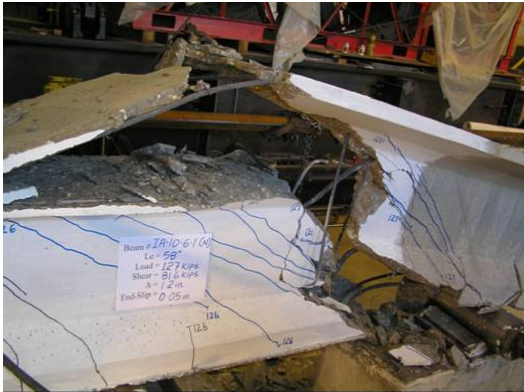
Photo showing shear failure at the opposite end for IA-10-6-1-N
