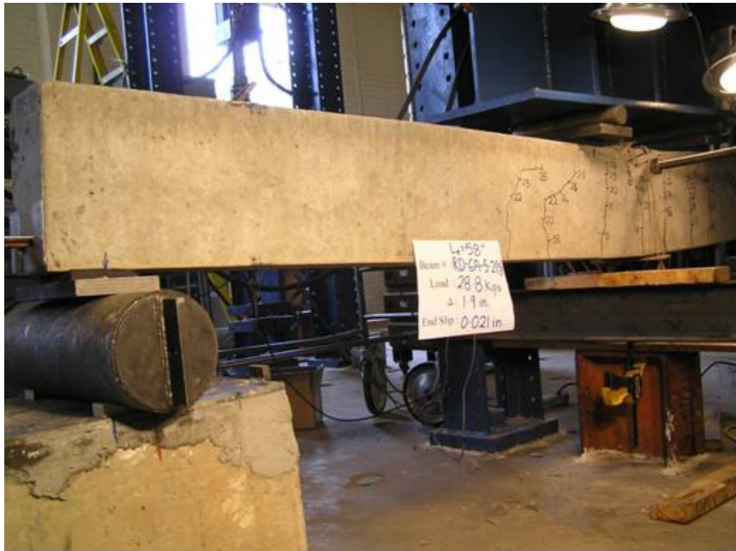
Cracking pattern for Beam RD-6A-5-2 being loaded at South end
