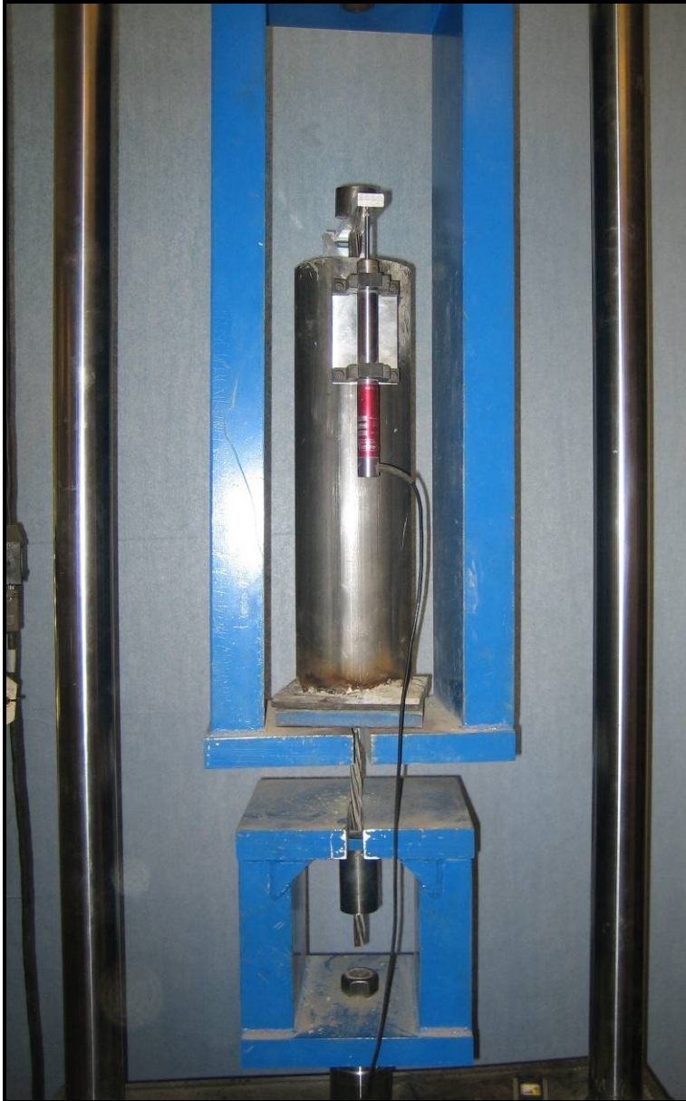
Figure 3.17: NASP Specimen on the Test Frame
