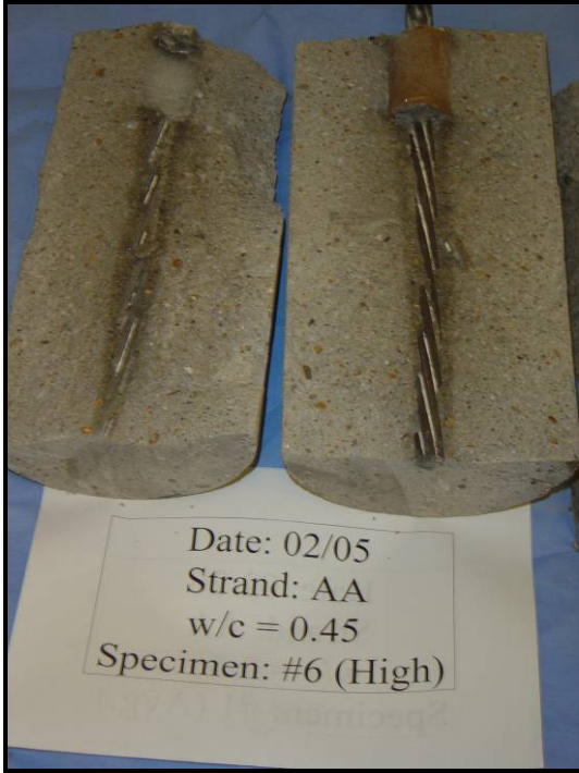
Figure 3.10: NASP Split Specimen for High value
