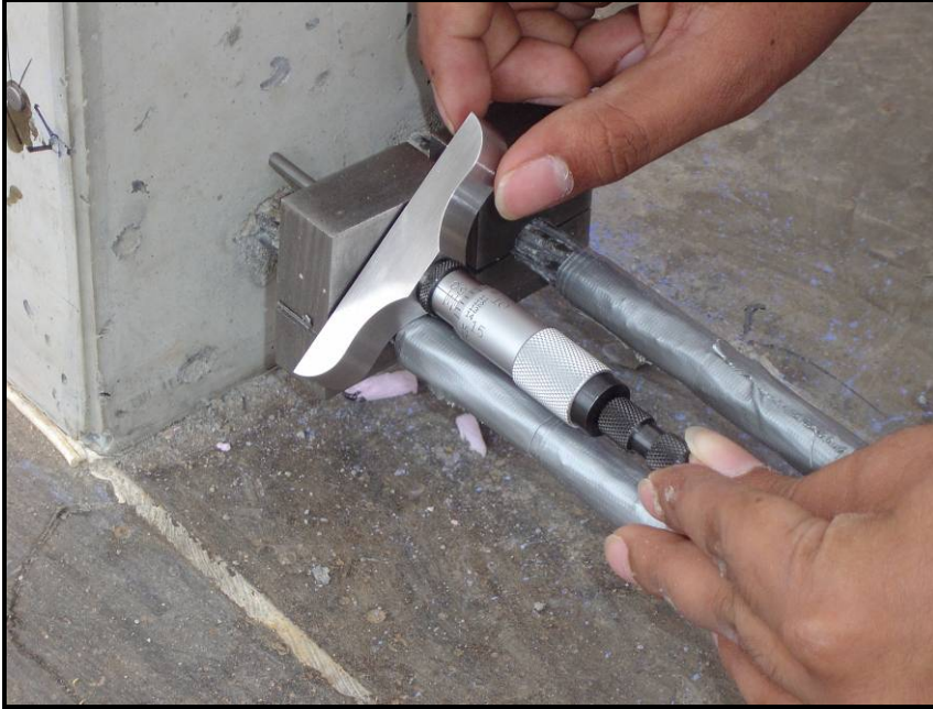
Figure 5.8: End Slip Measurement using analog micrometer
