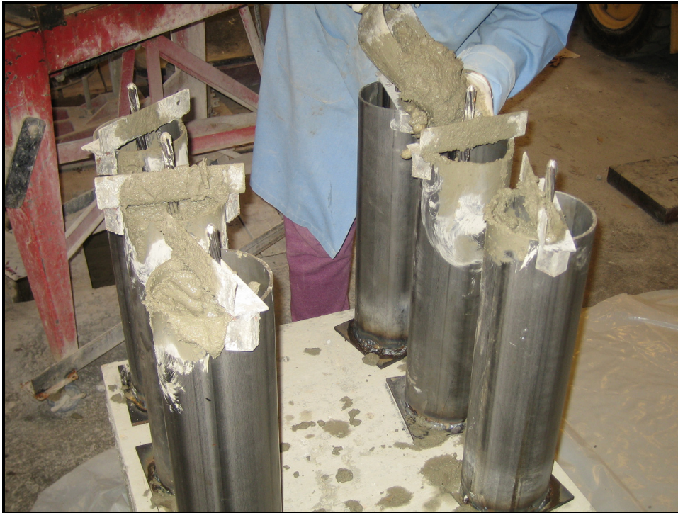
Figure 3.7: Preparing the NASP Specimens
