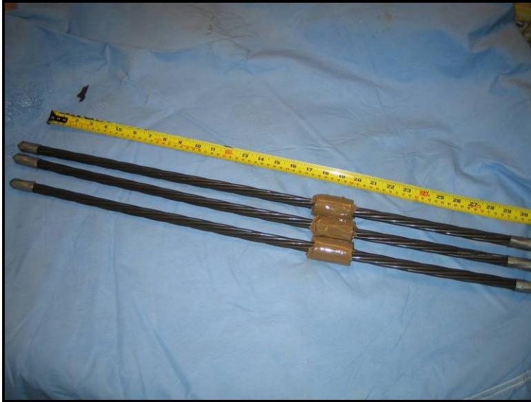
Figure 3.5: Specimen strands and bond breakers
