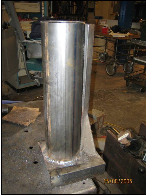
Figure 3.4: NASP Specimen Cylinder on the jig
