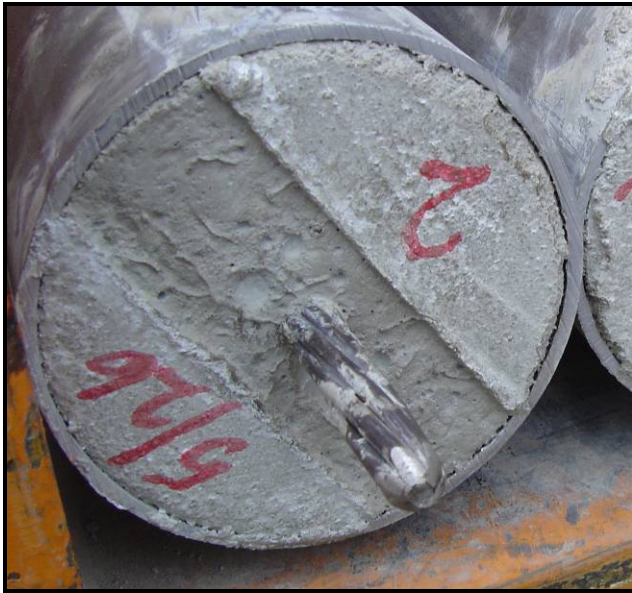
Figure 3.3: Strand embedded in NASP specimen
