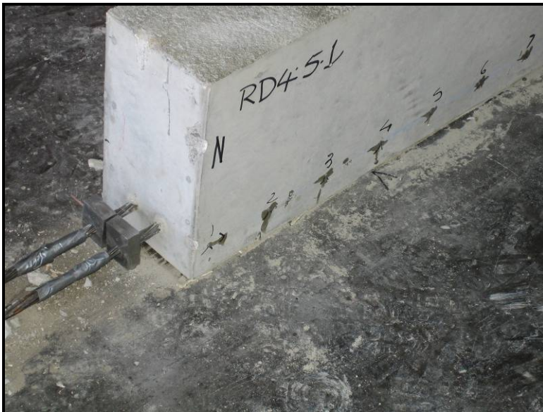
Figure 5.27: Moved RD4-5-1 after flame cutting
