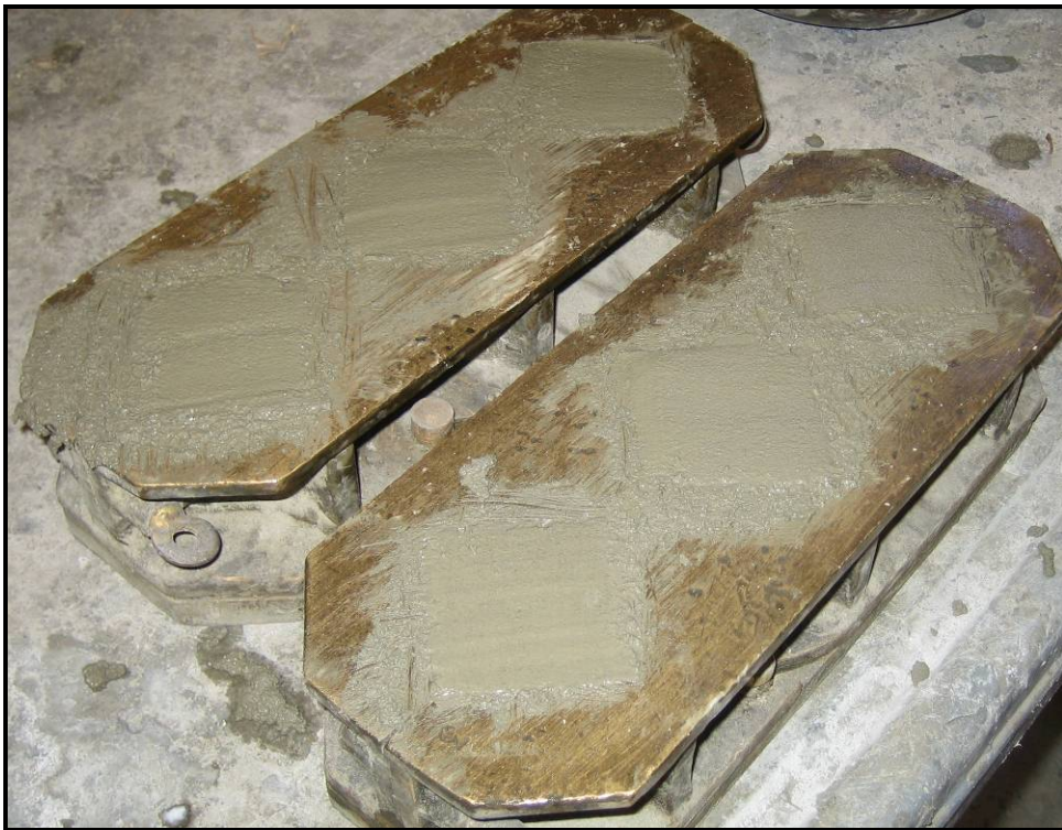
Figure 3.9: Fresh Mortar Cubes
