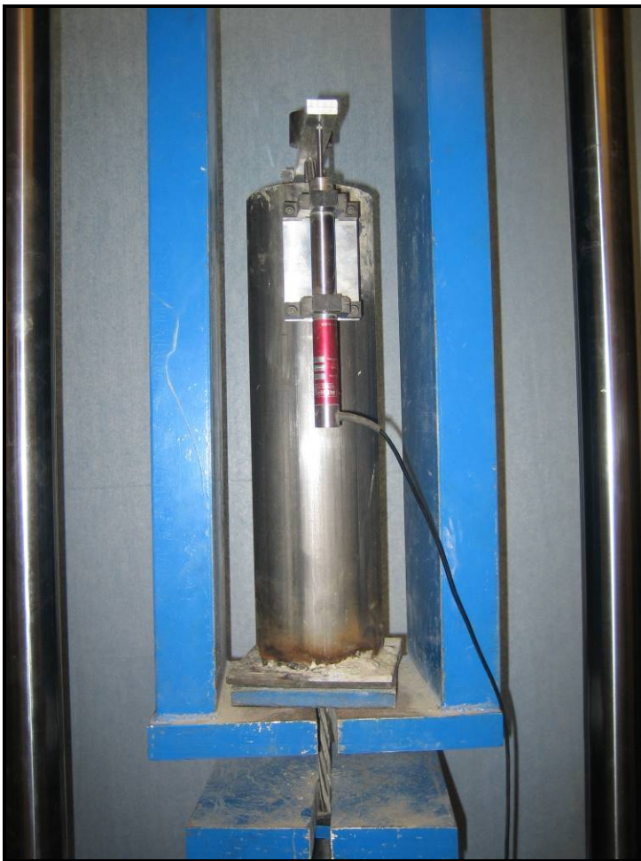
Figure 3.1: NASP Specimen on the loading frame
