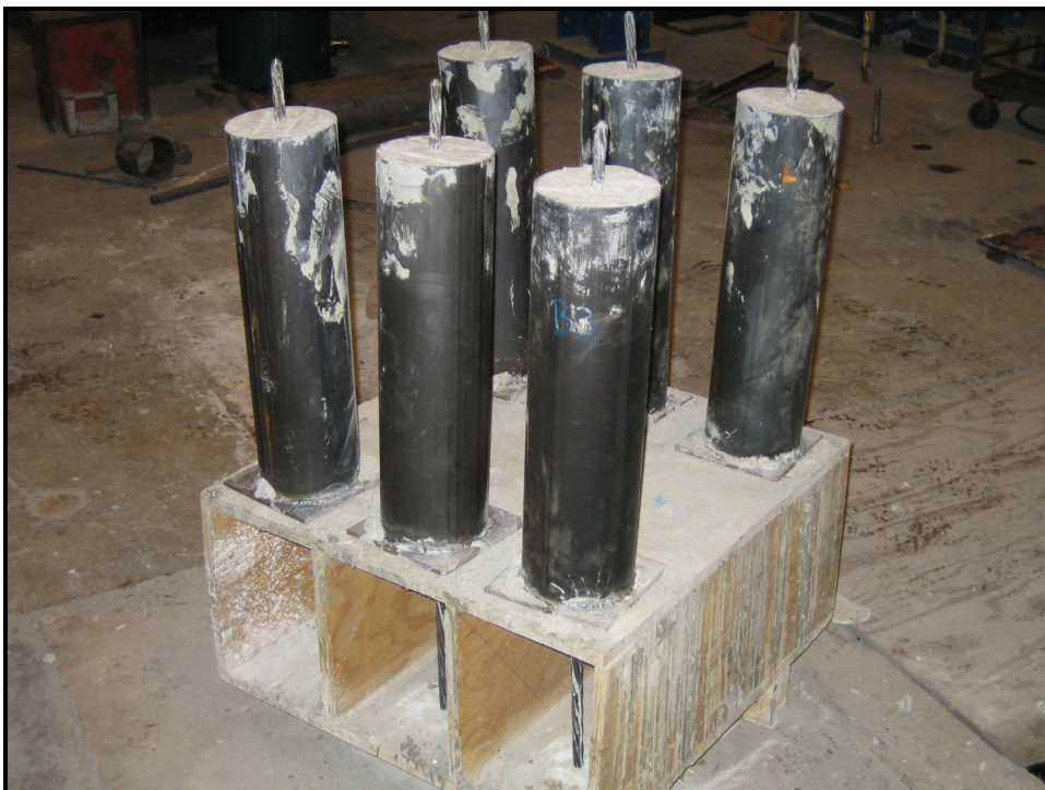
Figure 3.8: NASP Specimens on the wooden box after curing
