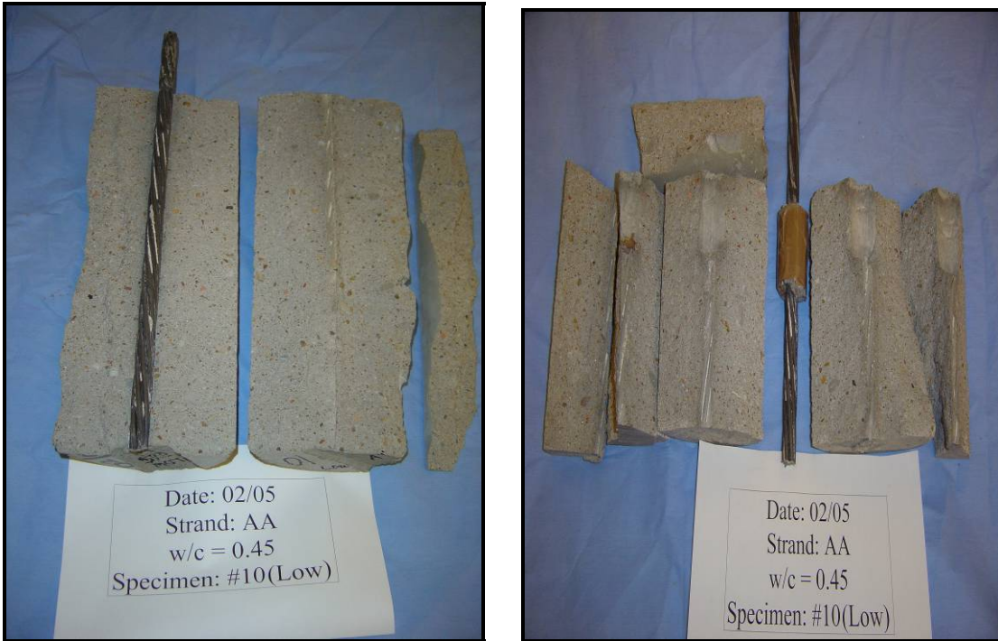
Figure 3.12: NASP Split Specimen for low value
