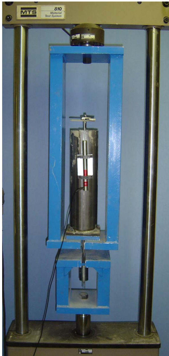
Figure. B.2. Typical Stiff Test Frame to Conduct NASP Bond Test
