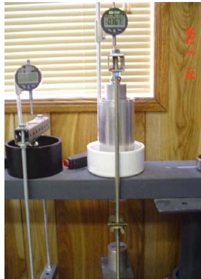
Figure 10 - Consolidating SPNC Direct Shear Specimen
