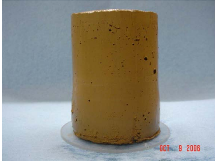
Figure 11 - Extruded SPNC Specimen
