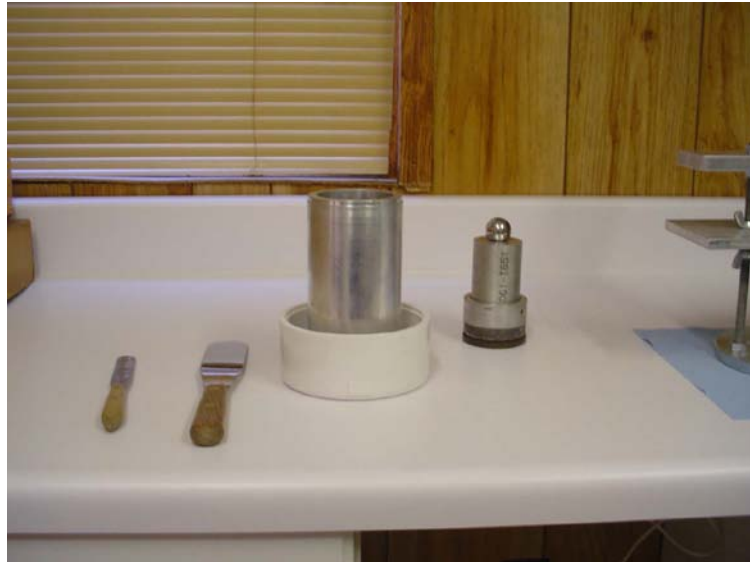
Figure 7 - SPNC Device for a 2.5" Direct Shear Specimen
