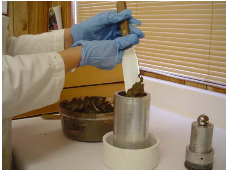
Figure 9 - SPNC Specimen Placement in Device
