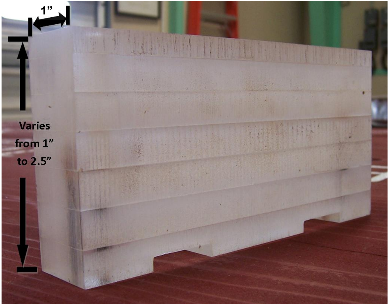
Figure 3.4 Typical sill dimensions.
