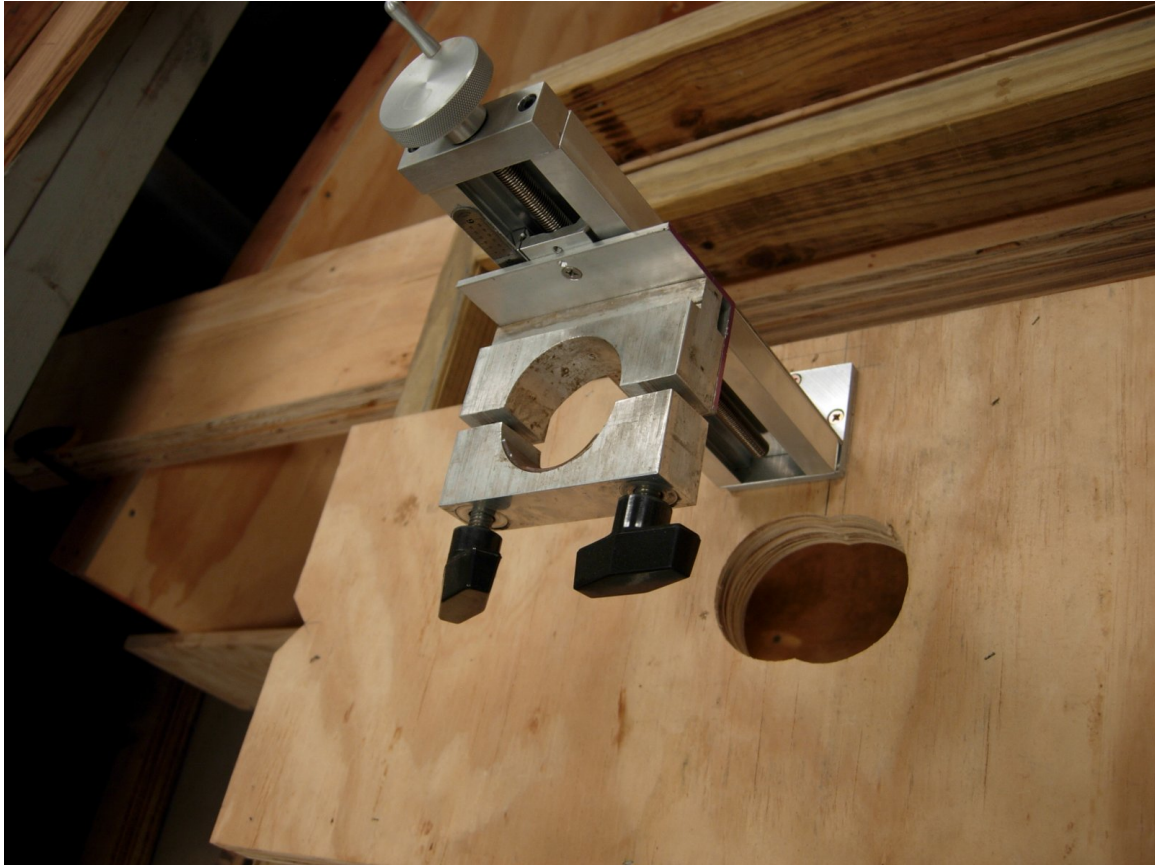
Figure 3.13 Acoustic Doppler Velocimeter (ADV) Mount over flume.
