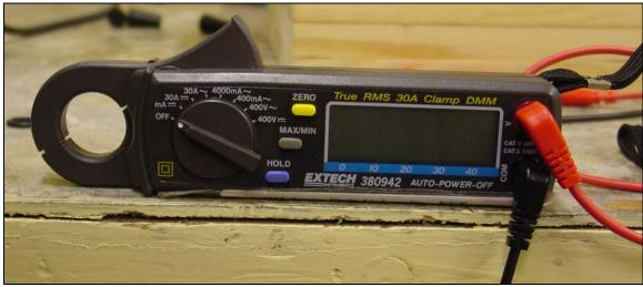
Figure 3.5 Clamp-on Ammeter
