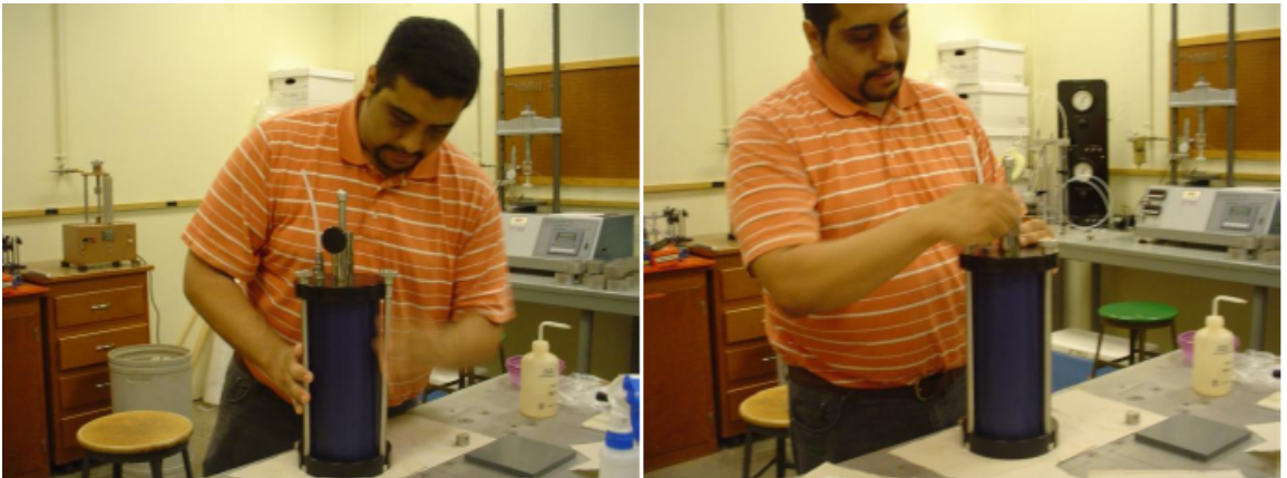
Figure 14—Assembly of Triaxial Cell
