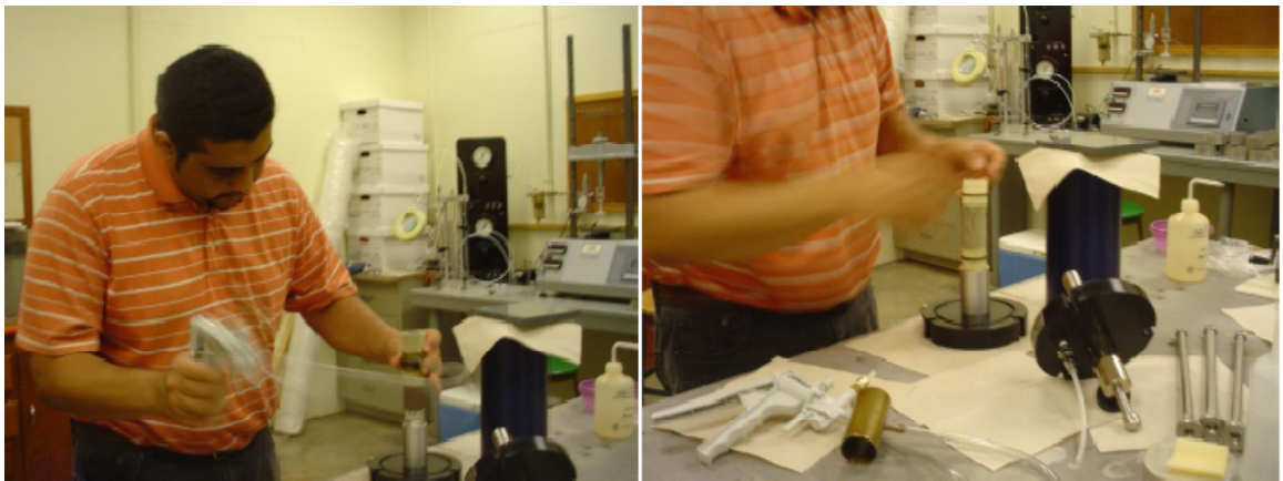
Figure 12--Installing Membrane on Samples Using Vacuum Pump
