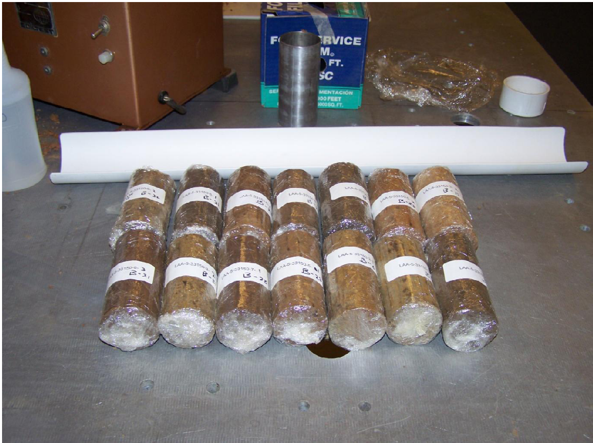
Figure 2 – Trimmed Samples in Length and Diameter
