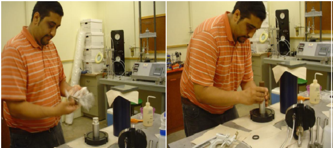
Figure 10--Mounting sample on Triaxial Base
