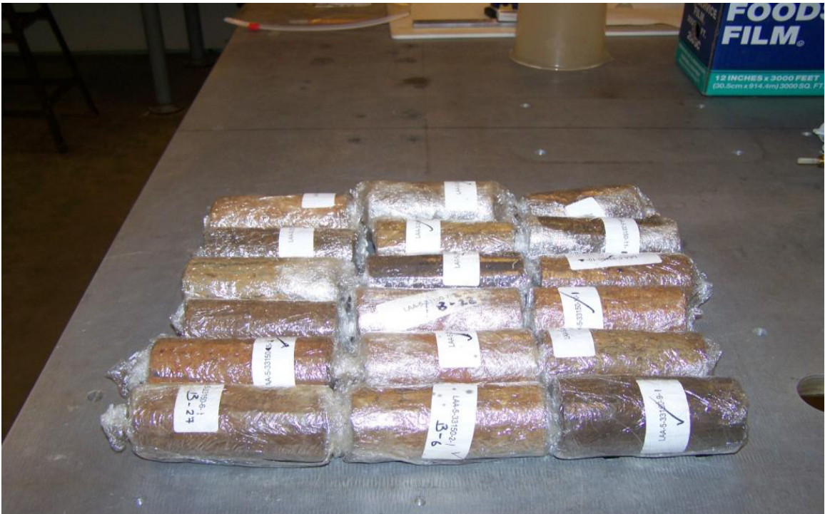
Figure 5--The Eighteen In-Situ Samples after shear Testing
