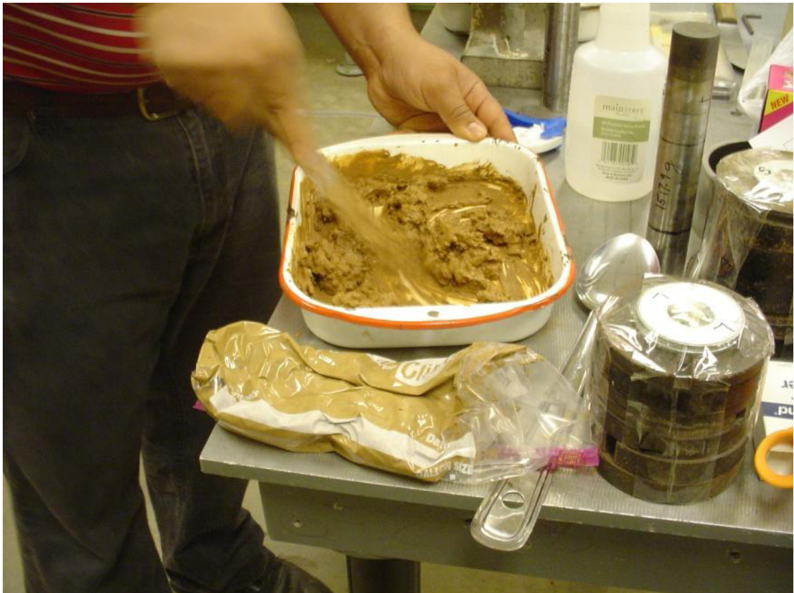
Figure 6--Slurry Mixing of Sample
