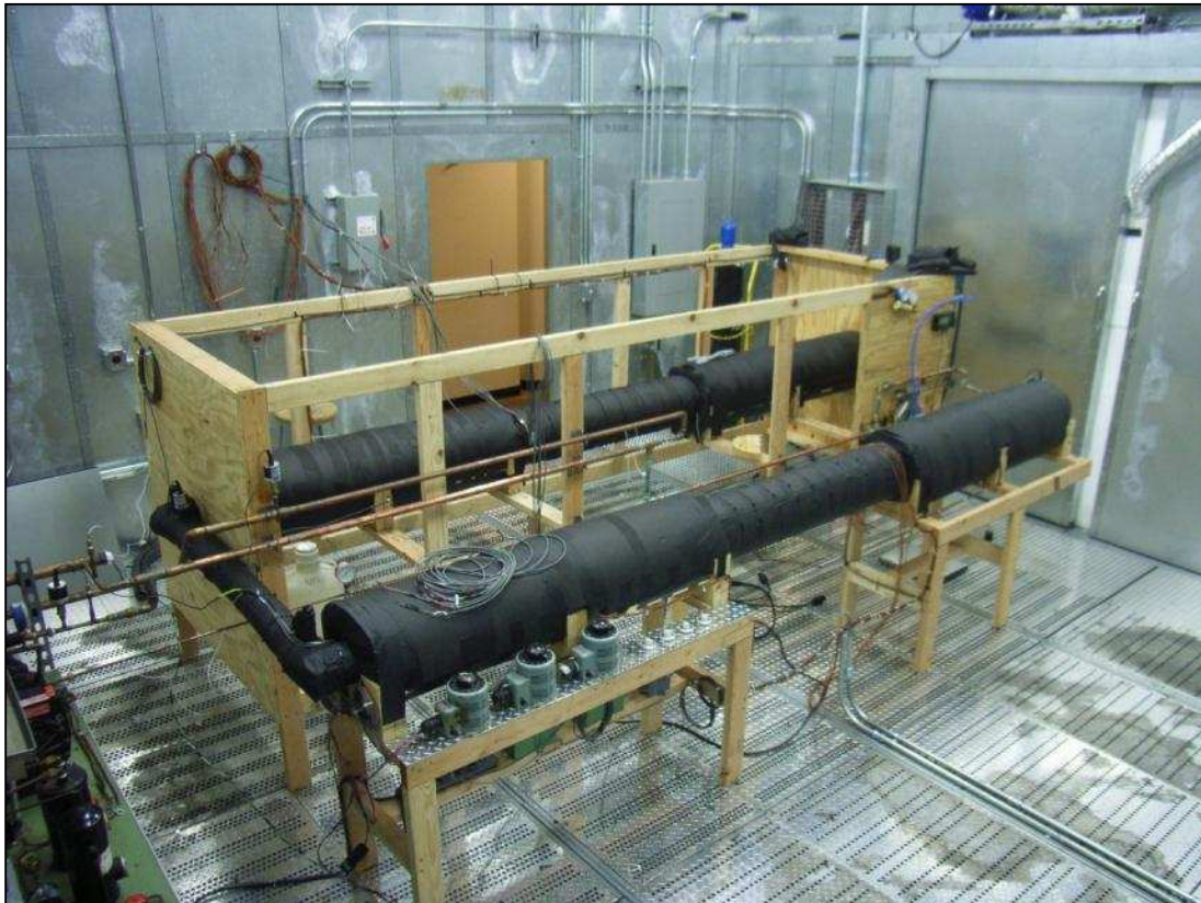
Figure 29 Pipe Insulation Tester Experimental Setup
