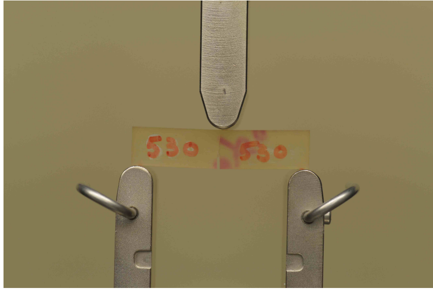
Figure 3.2: Fracture test carried on a specimen
