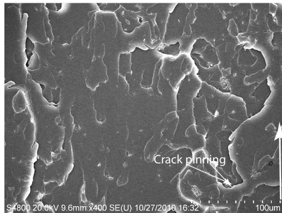
(a) fracture image showing the starter crack and the initiation of fracture region
