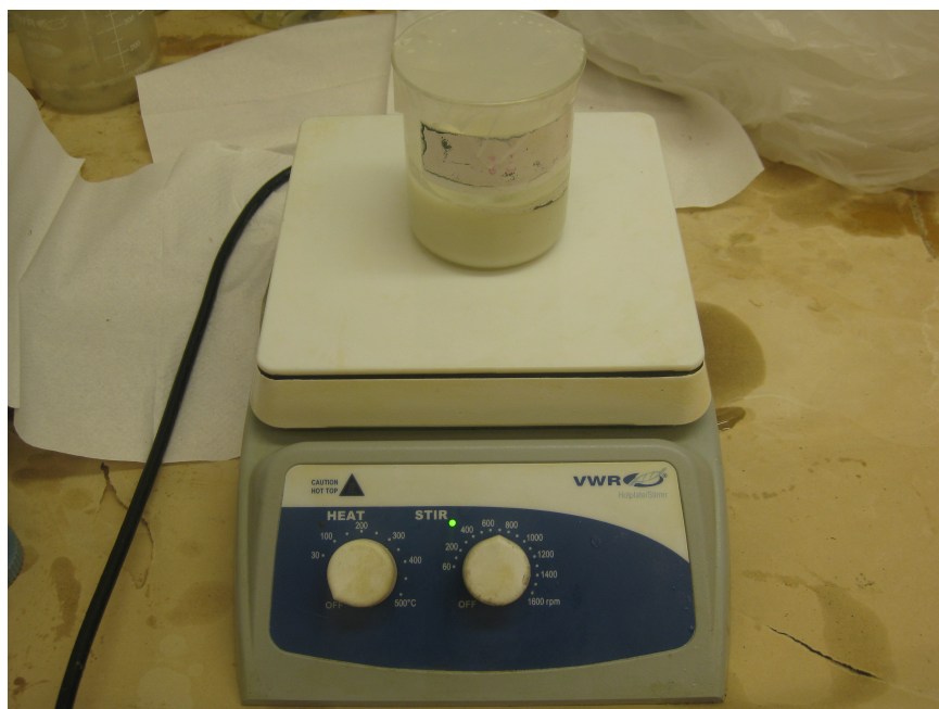
(a) Clay washed in methanol using magnetic stirrer
