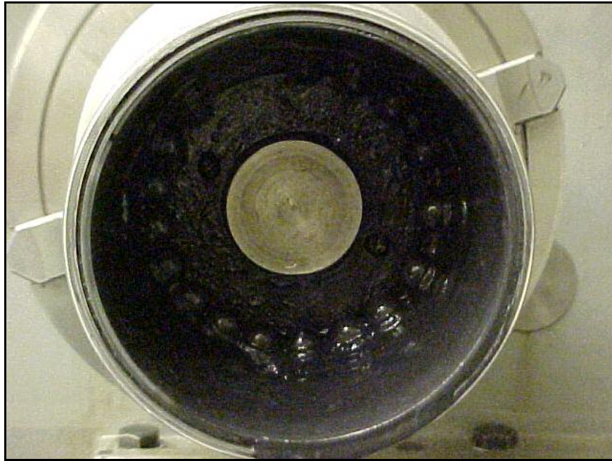
Figure 8.1.1 Full view photograph of the balls after the test run
