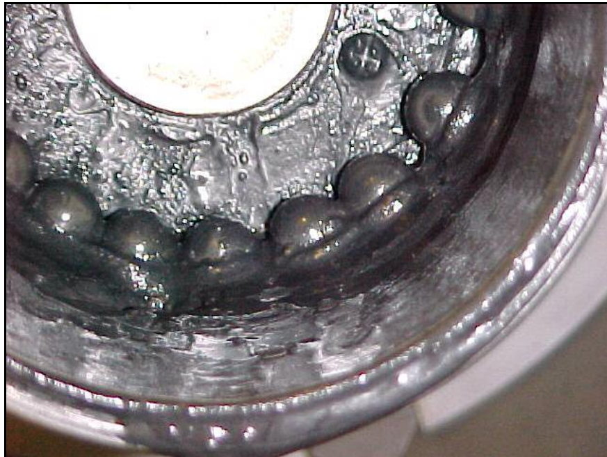
Figure 8.1.2 Photograph of balls immersed in abrasive slurry after the test run
