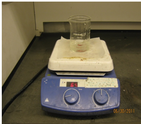
Figure 2.3: PVP/ethanol solution on a magnetic stirrer
