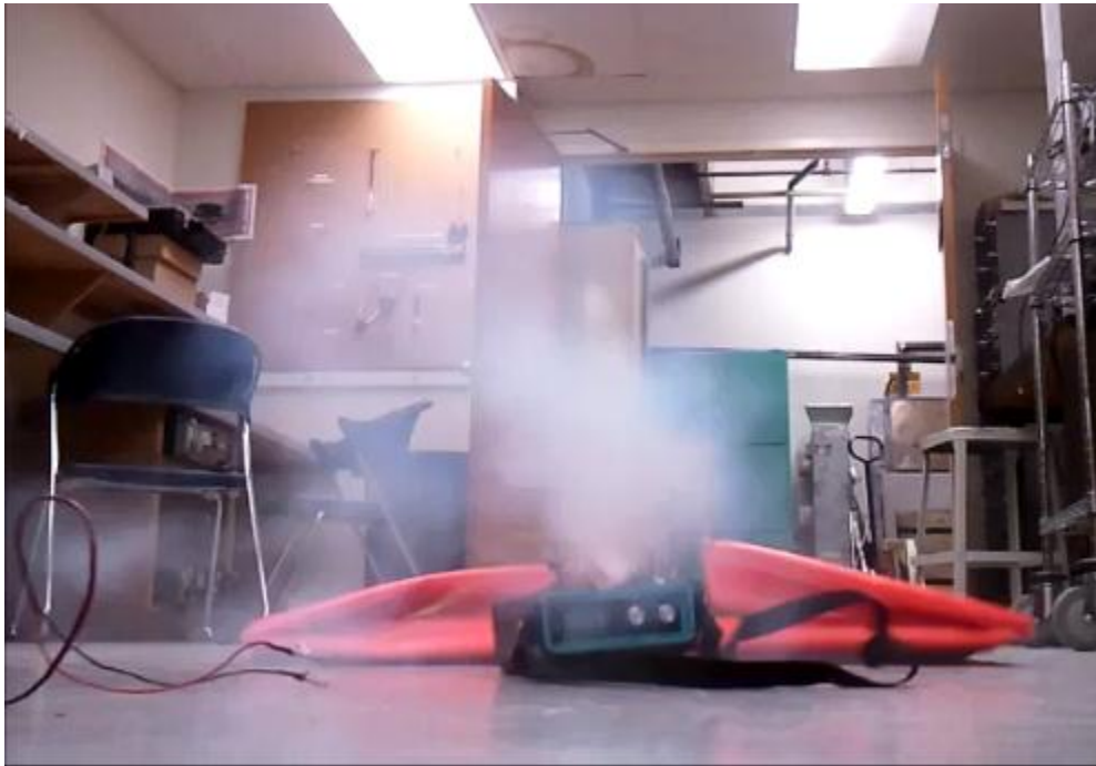
Figure 4.5.2: Early Inflation Test (Leak in the pressure gauge plumbing)
