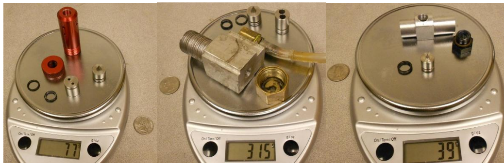
Figure 4.4.7: Pyro-Valve Weight Comparison
