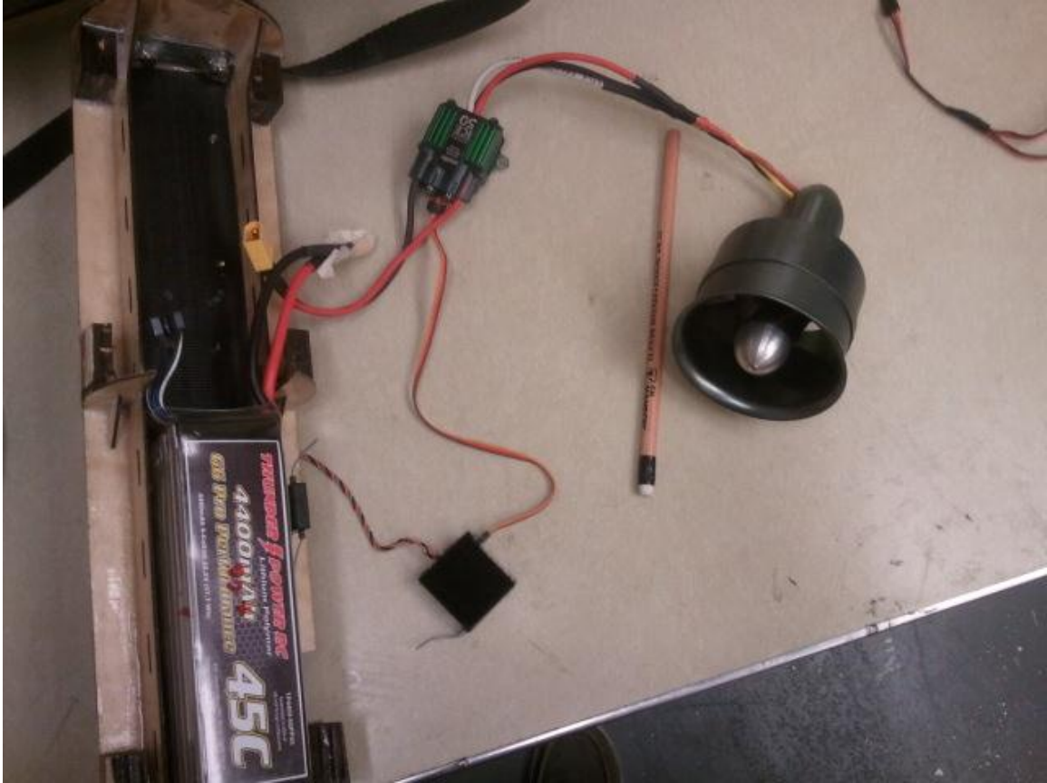
Figure 5.2.1: EDF Configuration Propulsion System
