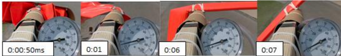
Figure 3.4.6: Z-Fold Dynamic Inflation Test
