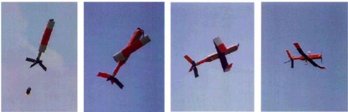
Figure 2.1.4: FLYRT Aircraft Deployment Sequence
