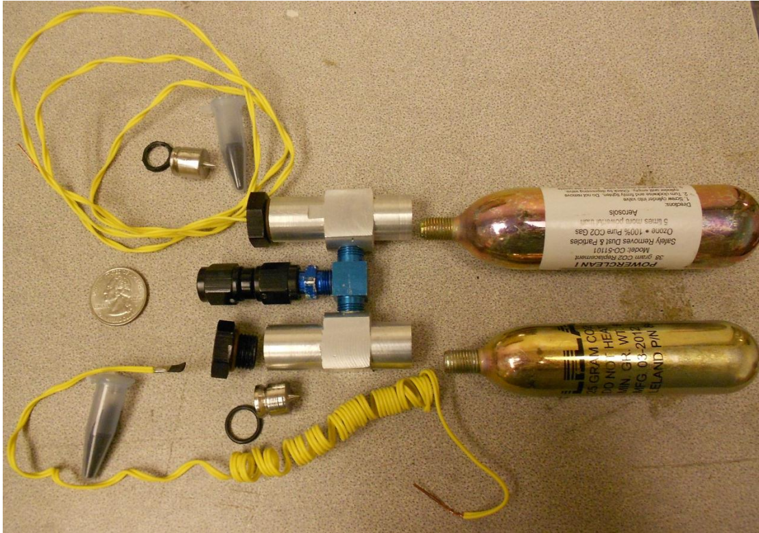
Figure 4.4.5: Completed Inflation System
