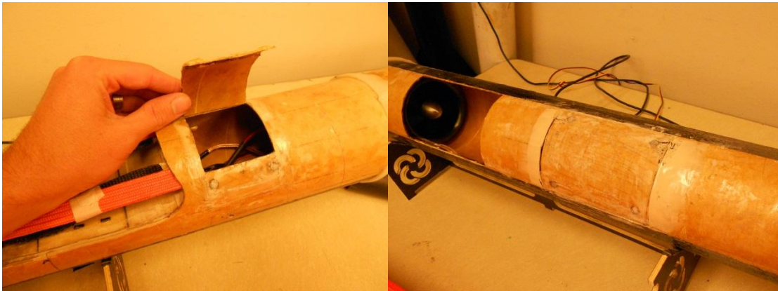
Figure 5.4.1 Access Hatches on Aircraft
