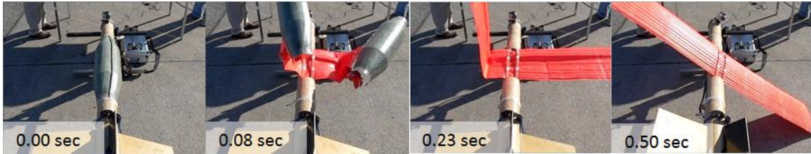
Figure 6.1.1: Wing Deployment Test
