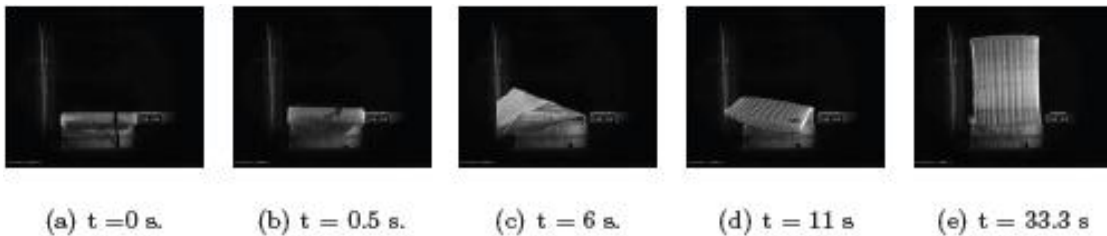
Figure 2.3.1: Deployment Test with Slow Inflation
