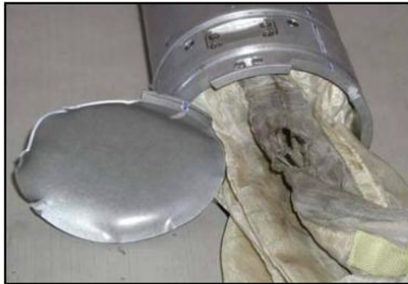
Figure 2.2.2.3: Gas Generator Destroyed Ballute [9]
