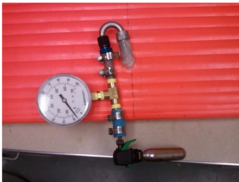
Figure 4.3.3: Wing Volume Testing with Co 2 Cartridges
