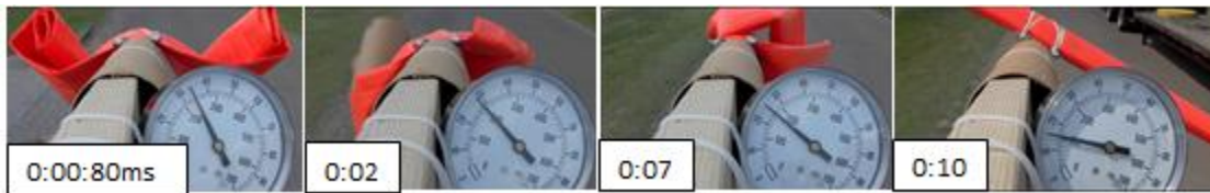
Figure 3.4.8: Roll Method Dynamic Inflation Test
