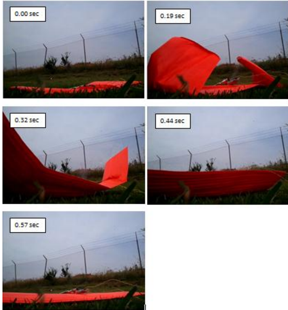
Figure 4.5.3: Inflation Test Time-lapse
