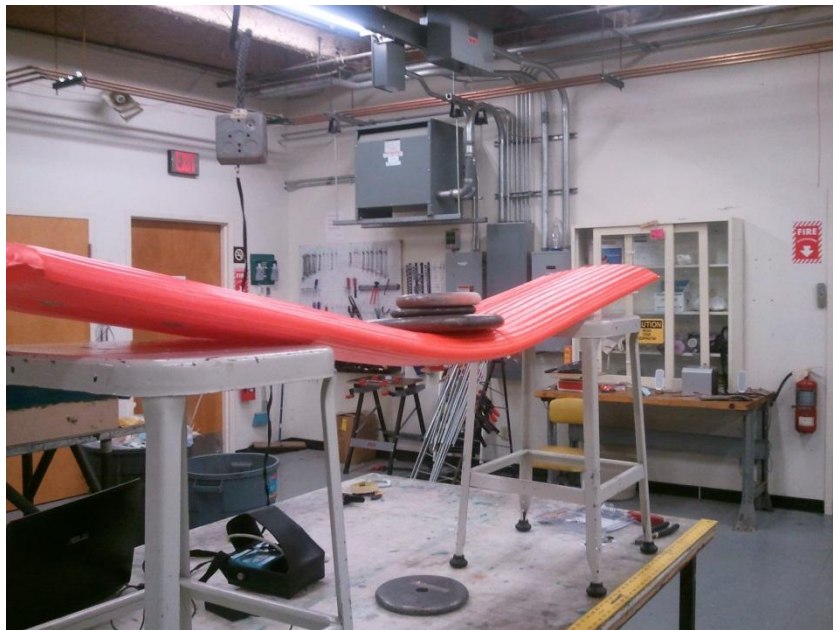
Figure 3.3.1: Inflatable Wing Bending Test Experimental Setup
