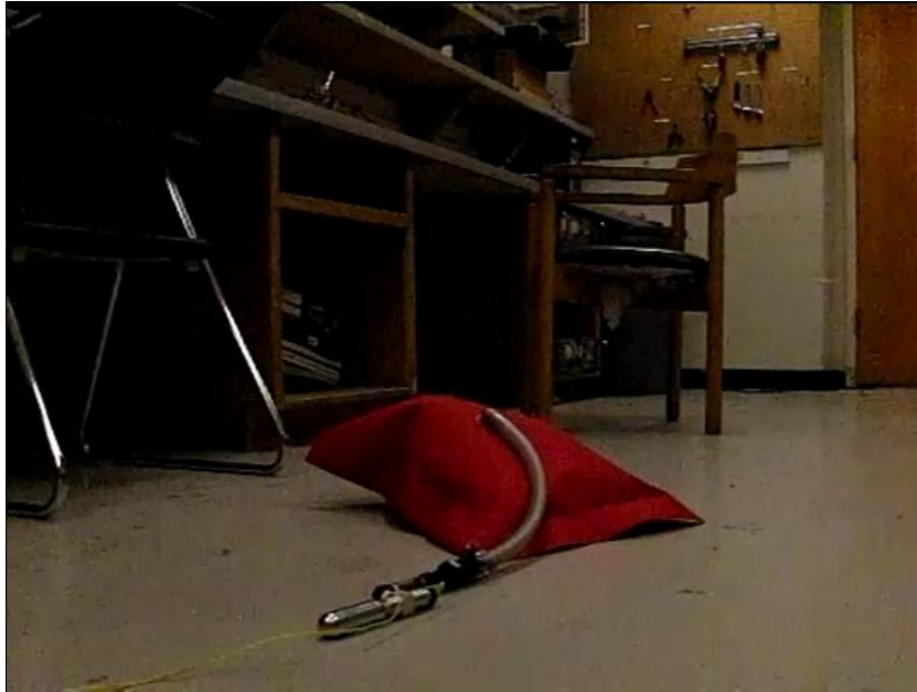
Figure 4.5.1: Inflation Test on Inflatable “Pillow”
