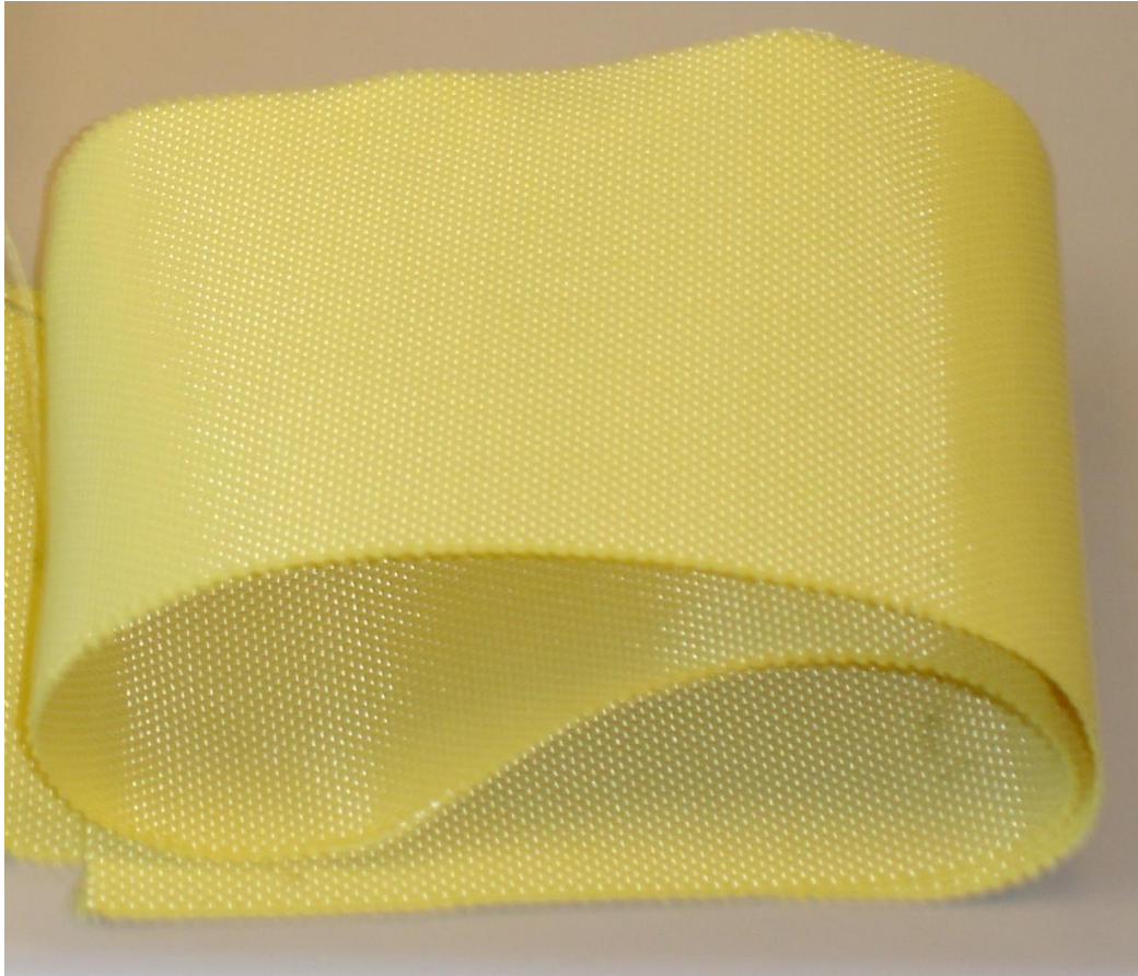
Figure 13: Dry woven Kevlar used for wrapping around the armor plate.
