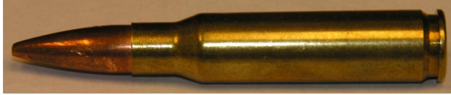
Figure 26: 0.308 Winchester bullet: the copper covered lead core of the bullet has a diameter of 7.9 mm (0.31 inch), a length of 27.6 mm (1.09 inch), and weighs 11.66 g (0.03 lb). The bullet has a muzzle velocity of approximately 798.6 m/s (2620 ft/s).
