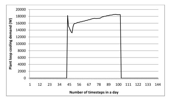
Fig 6.3 Plant loop cooling demand for design day
