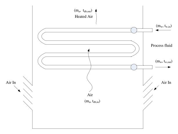
Fig 1.1 Schematic of dry fluid cooler
