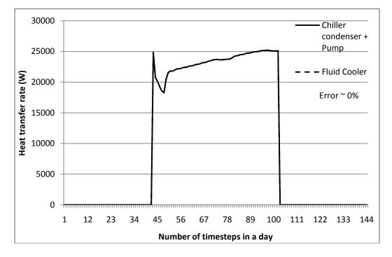
Fig 6.11 Condenser and pump heat addition vs. Fluid cooler heat transfer rate
