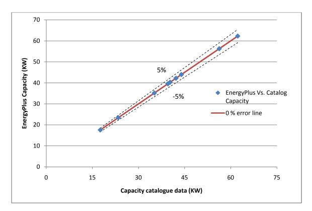
Fig. 5.1 Catalogue data Vs EnergyPlus capacity (KW)
