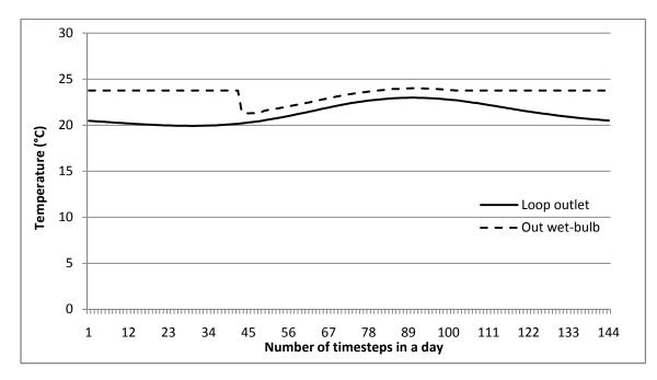
Fig 6.13 Air wet-bulb and loop outlet temperature on the design day
