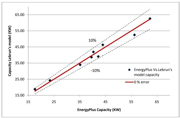
Fig. 5.3 EnergyPlus Vs Lebrun model capacity (KW)
