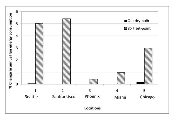
Fig 4.1 Comparison of % change in dry fluid cooler fan energy consumption due to change in
