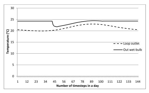
Fig 6.16 Air wet-bulb and loop outlet temperature on the design day
