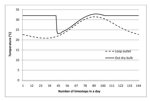
Fig 6.9 Air dry-bulb and loop outlet temperature on the design day
