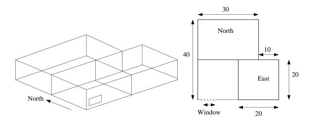
Fig 6.2 Isometric and plan views of the building
