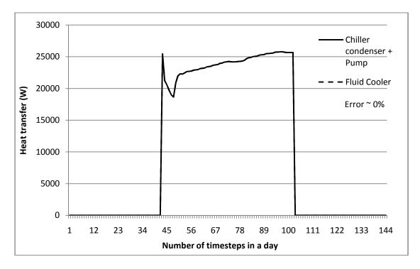
Fig 6.4 Condenser and pump heat addition vs. Fluid cooler heat transfer rate
