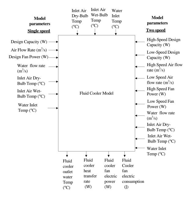
Fig 3.4: Information flow chart for design capacity method of fluid cooler models in EnergyPlus
