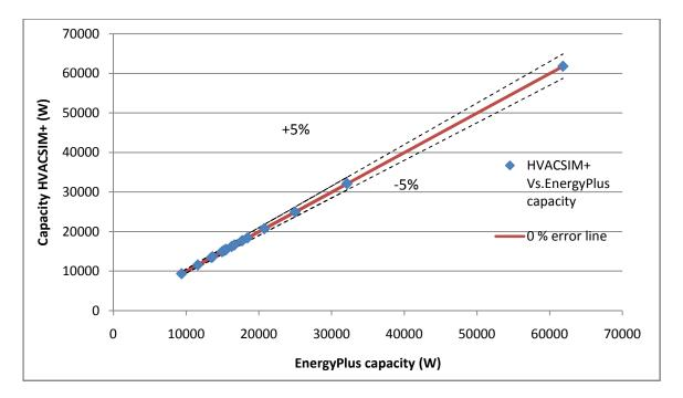
Fig. 5.2 EnergyPlus Vs HVACSIM+ capacity (W)
