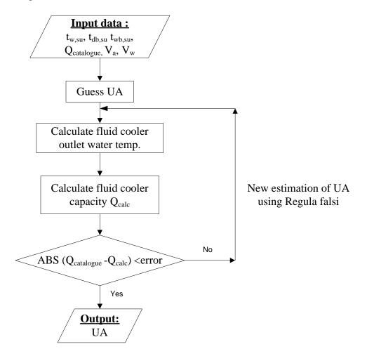
Fig 3.5 Flow chart for UA calculation method used by EnergyPlus
