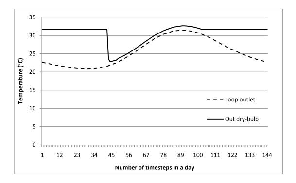
Fig 6.6 Air dry-bulb and loop outlet temperature on the design day
