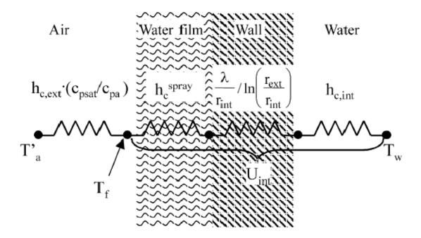
Fig 2.2 Heat transfer scheme of closed circuit cooling tower
