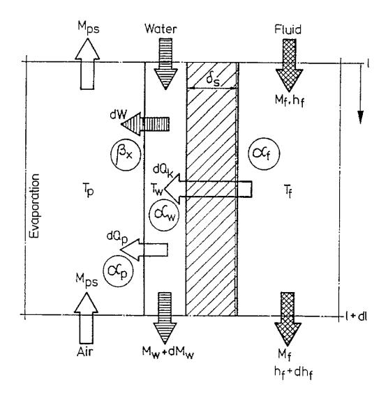
Fig 2.1 Heat exchange scheme of evaporative fluid cooler
